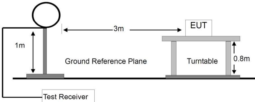
For Radiated Emission 30-1000MHz
