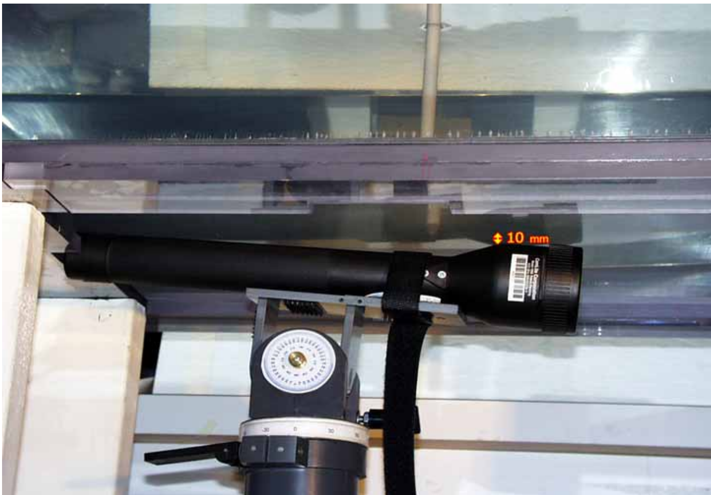
< Side of D.U.T. parallel to the phantom, 10 mm separation distance >
