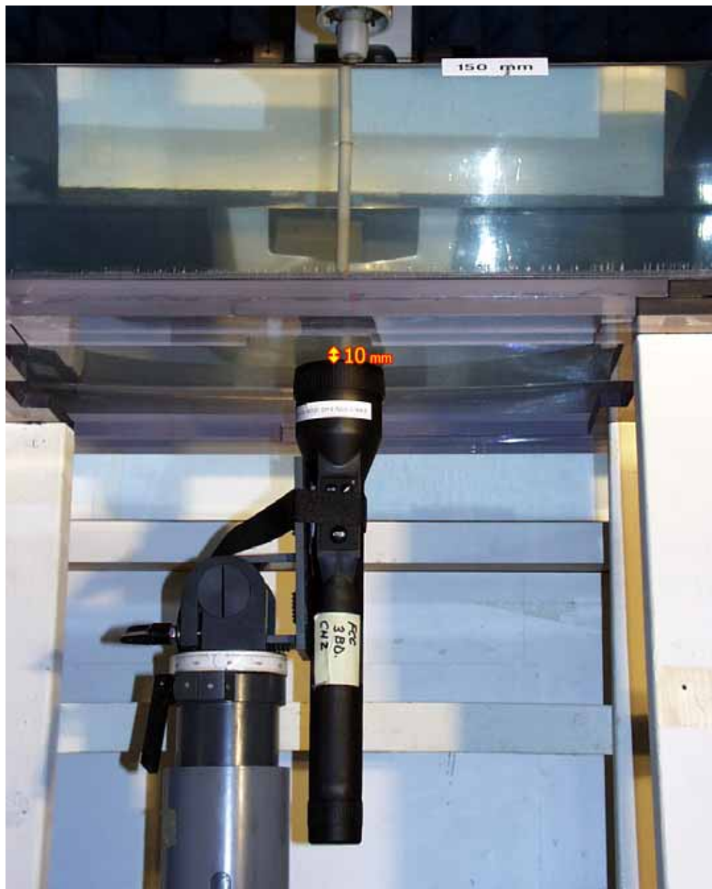
< Front of D.U.T. pointed toward the phantom, 10 mm separation distance >
