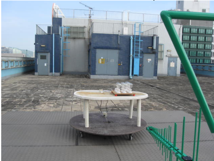
Radiated Emission Test Set Up
