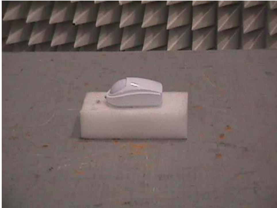
Radiated Emissions Test Configuration
