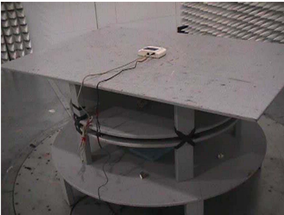
Radiated Emissions Test Configuration
