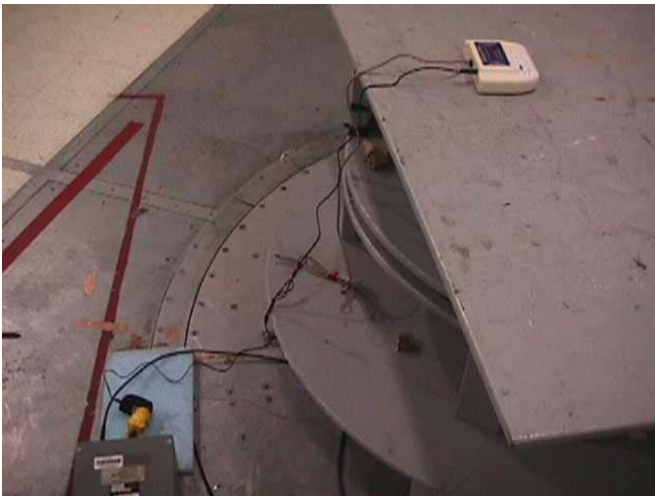
Conducted Emissions Test Configuration
