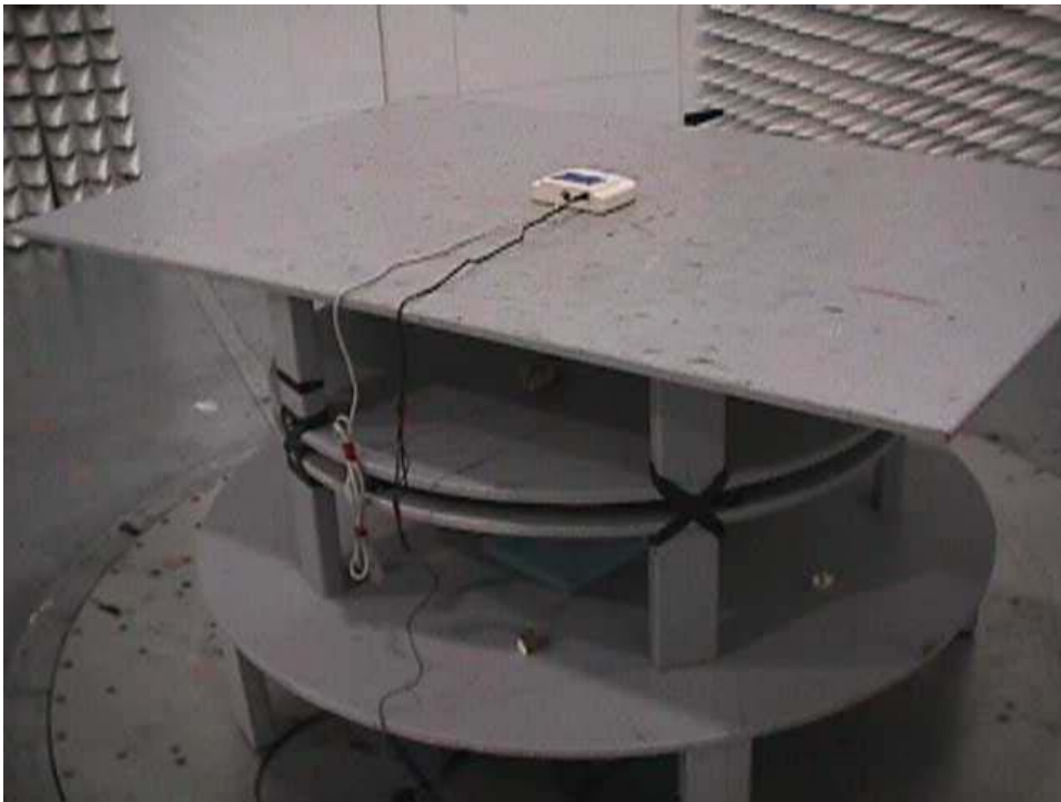
Radiated Emissions Test Configuration
