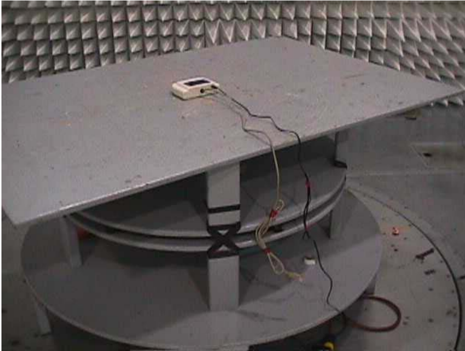
Radiated Emissions Test Configuration
