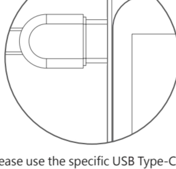
Please use the specific USB Type-C cable with the certified DC5V---1A adaptor to charge.
