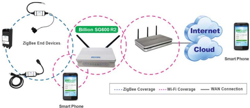
The Billion BILLION SG600R2, ZigBee Wireless Smart Energy Gateway, is a TCP/IP based ZigBee/Wi-Fi appliance designed for users to enjoy real-time power management. Integrated with ZigBee wireless technology, the BILLION SG600R2 can communicate wirelessly with Billion ZigBee-enabled smart device, like SG3015-Tx meter and SG110-A Temperature / Humidity sensor.
