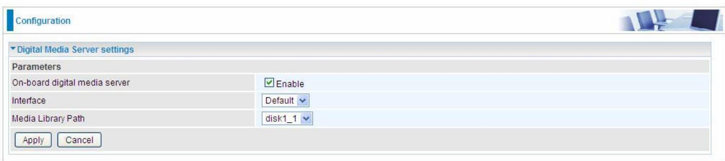
The screenshot shows a configuration interface for a DLNA server. The top bar has a 'Configuration' tab and a small icon. The main area is titled 'Digital Media Server settings' with a 'Parameters' section. It includes three fields: 'On-board digital media server' with a checked 'Enable' checkbox, 'Interface' set to 'Default', and 'Media Library Path' set to 'disk1\_1'. At the bottom are 'Apply' and 'Cancel' buttons.
