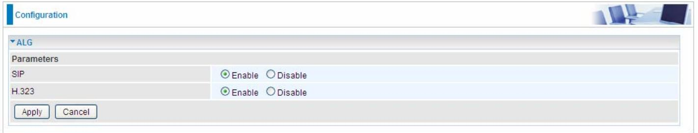
**SIP:** Enable the SIP ALG when SIP phone needs ALG to pass through the NAT. Disable the SIP when SIP phone includes NAT-Traversal algorithm.
