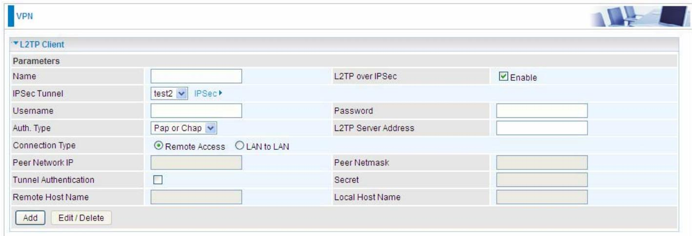
The screenshot shows the 'L2TP Client' configuration page with the 'Enable' checkbox checked. The other fields are identical to the previous screenshot.
