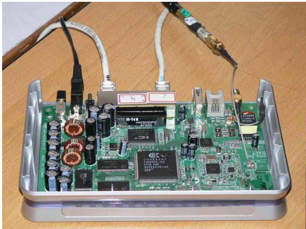
**POWERLINE CONDUCTED EMISSIONS MEASUREMENT SETUP**
