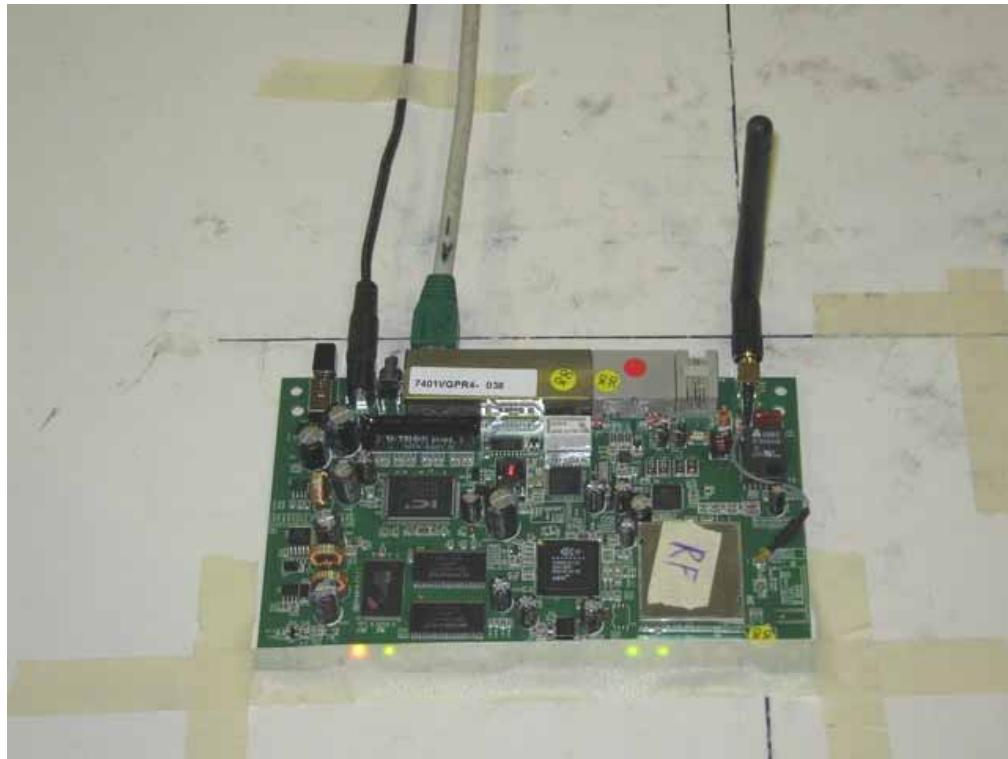
**ANTENNA PORT CONDUCTED RF MEASUREMENT SETUP**
