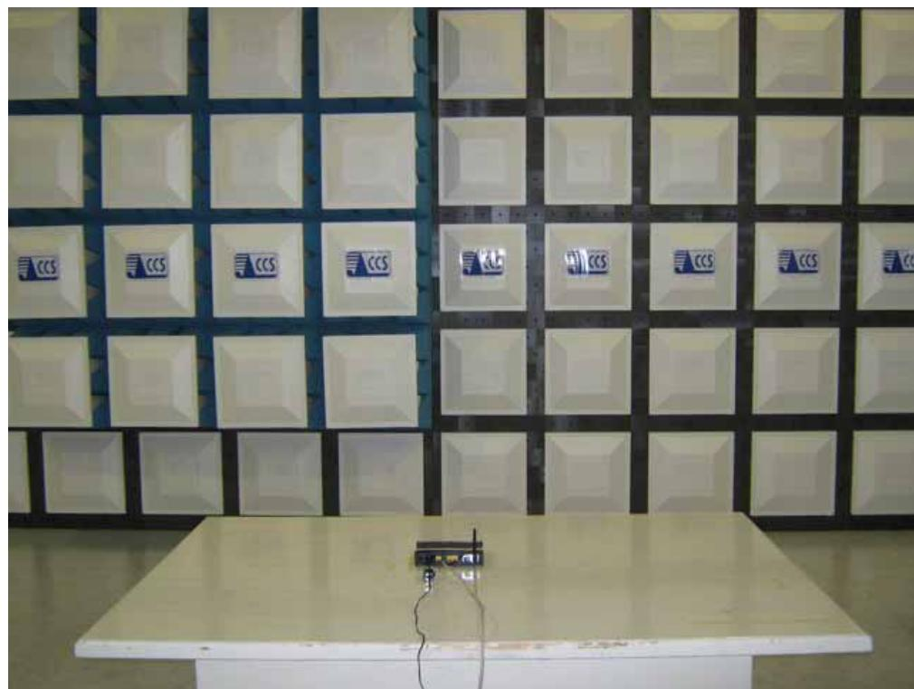
**ANTENNA PORT CONDUCTED RF MEASUREMENT SETUP**
