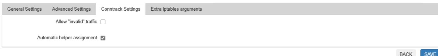
**Allow Invalid Traffic:** is a setting in the firewall's configuration that determines whether packets classified as "invalid" by the connection tracking system should be allowed through the firewall.
