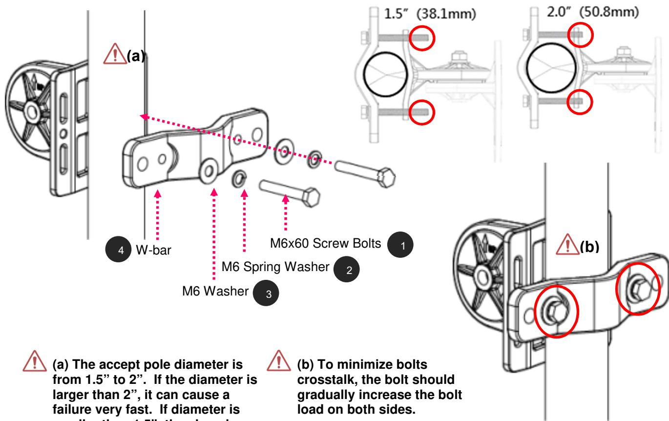
**!** (a) The accept pole diameter is from 1.5" to 2". If the diameter is larger than 2", it can cause a failure very fast. If diameter is smaller than 1.5", the clamping force might be insufficient in holding the device to the pole.
