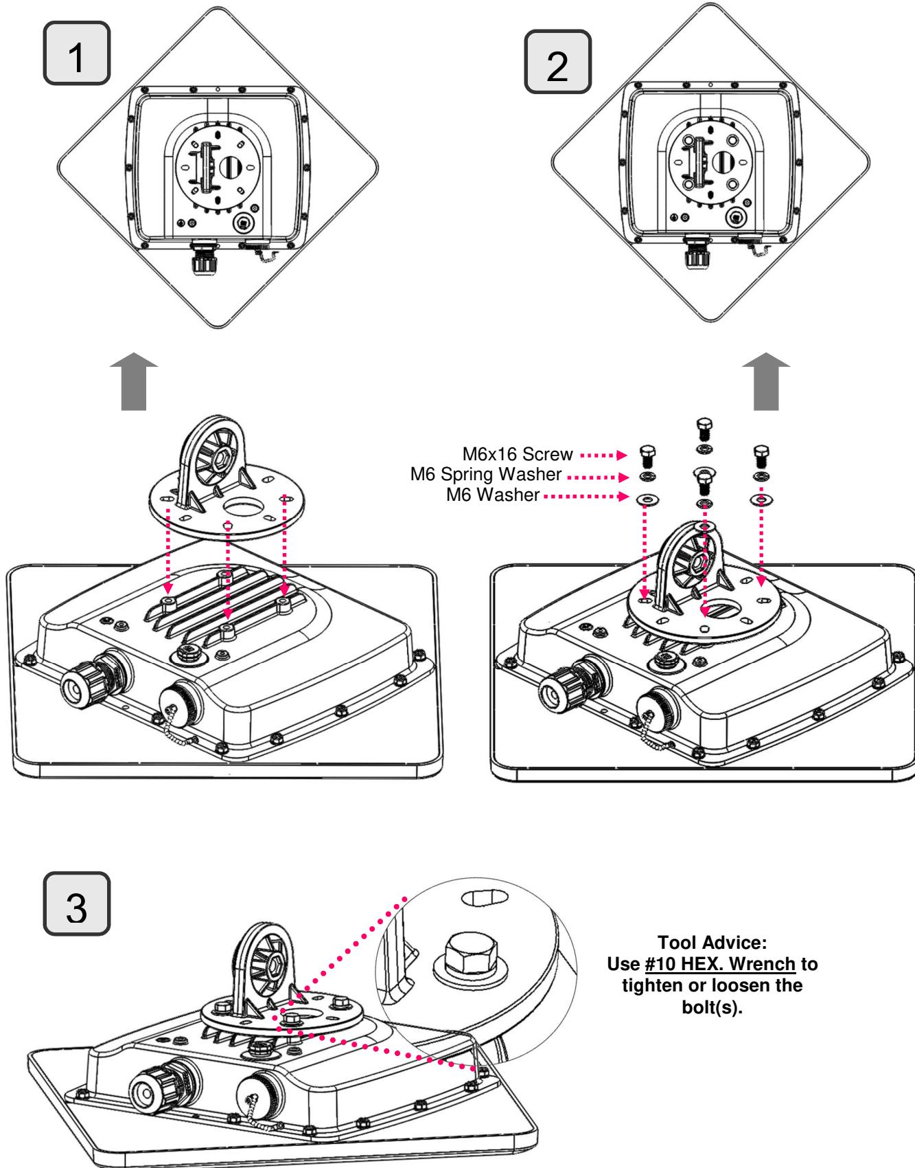
**Note:** The flexible mounting kit can be adjusted in multiple angles to align with the base station for higher efficiency.
