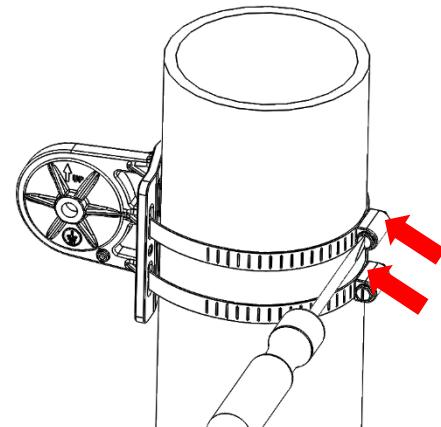
Fix the T-formed Bracket to the pole by using the supplied stainless hose clamps. Use a flat-head screwdriver to turn the head of the screw clockwise to tighten it.
