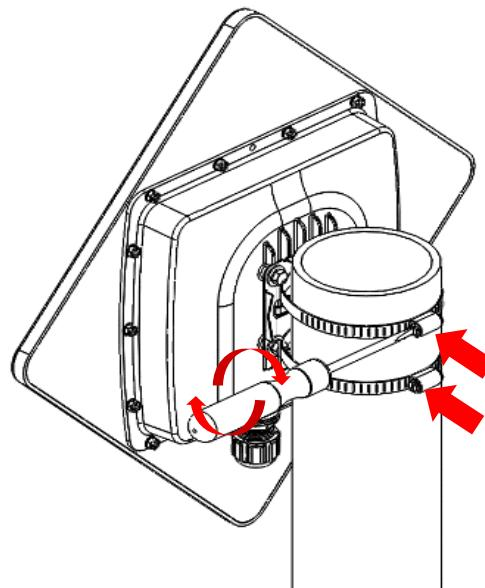
Fix the stainless-steel bracket to the pole by using the supplied stainless hose clamps (1" ~ 3"). Use a flat-head screwdriver to turn the head of the screw clockwise to tighten it.
