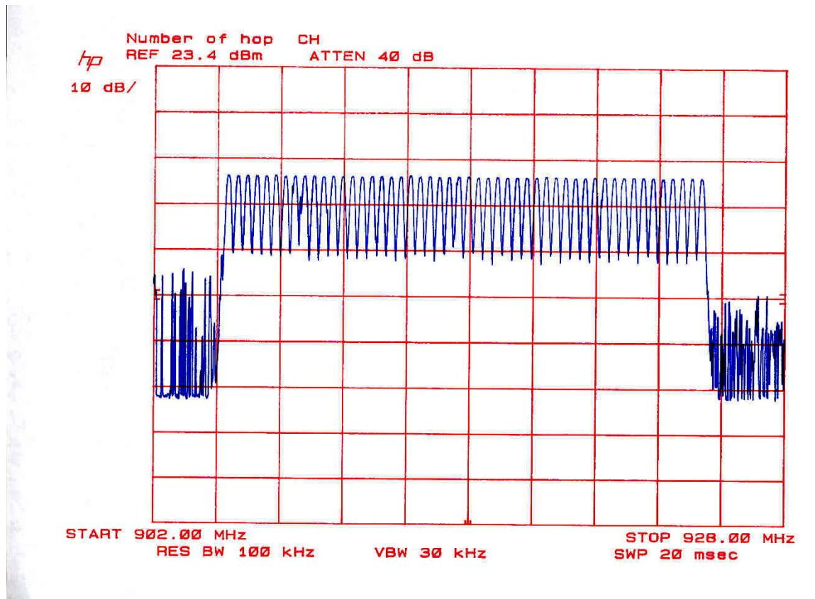
**Channel separation: 400 kHz (minimum separation = 25 kHz or 20 dB BW)**
