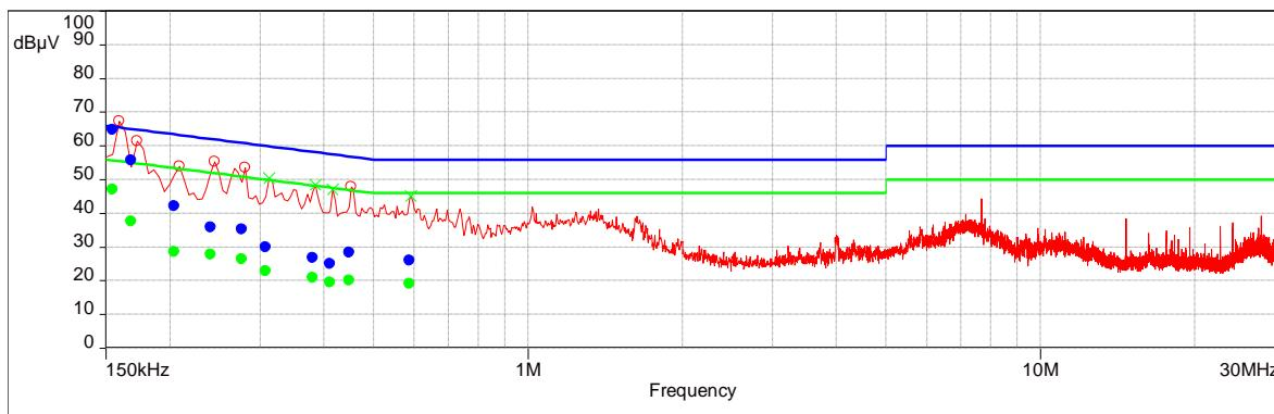
test name Single Phase Under 20 Amp\_150kHz to 30 MHz ESCI\_120VAC 60Hz\_Worst-Case output power-modulation-channel Time ate 19/8/2024 17:12
