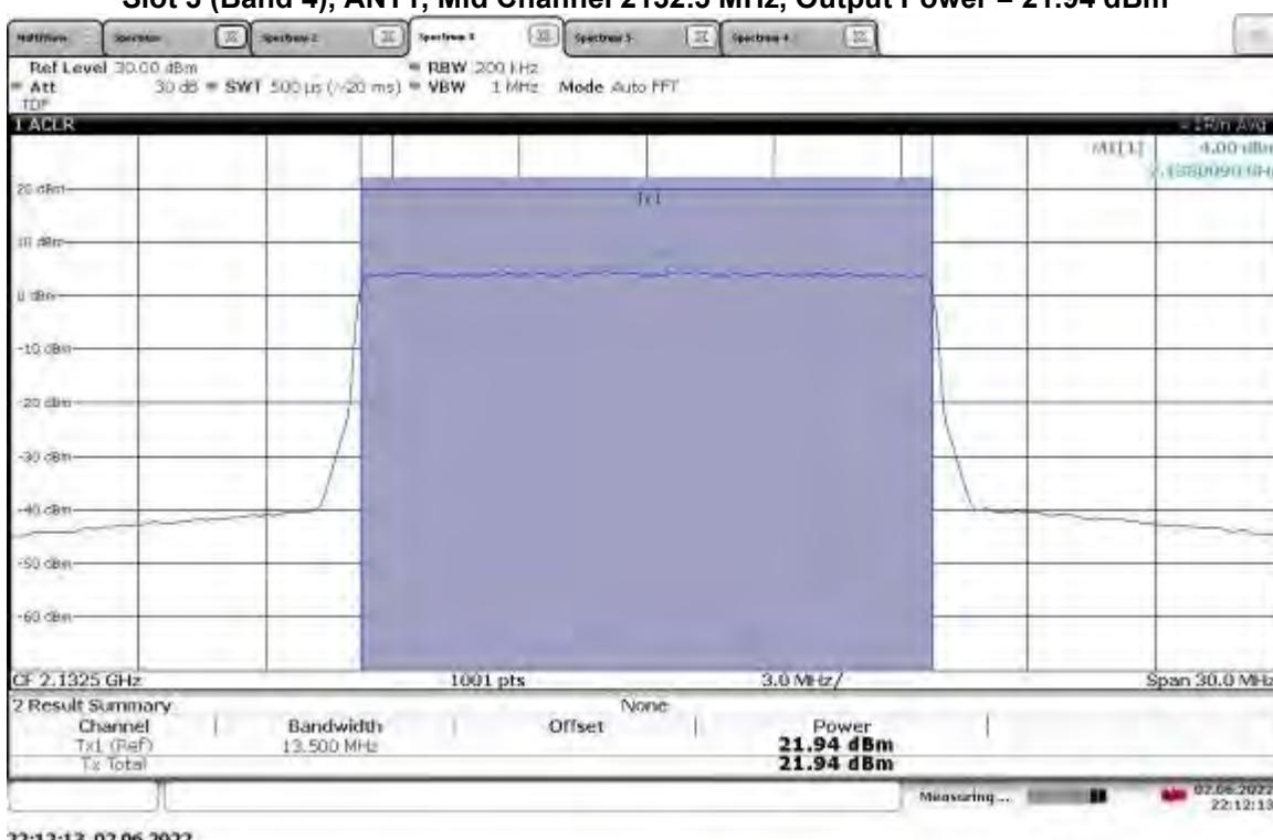
**TM3.1a-256QAM\_15 MHz Bandwidth**
