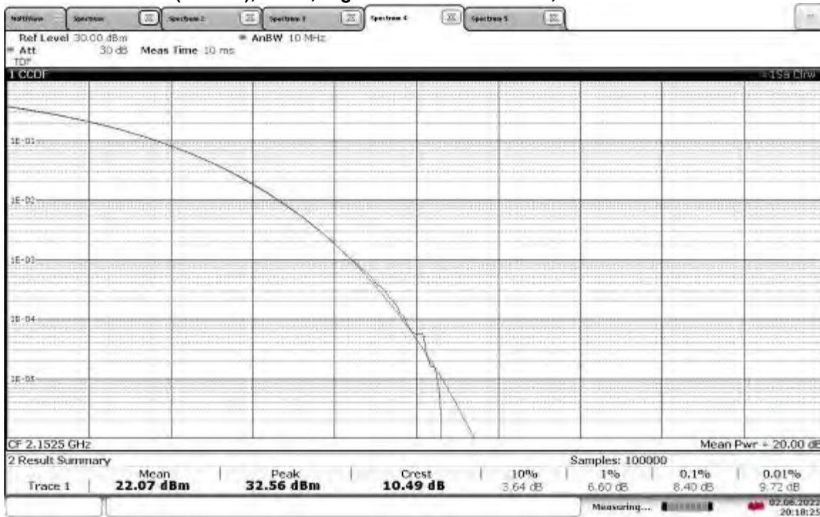
**TM3.1a-256QAM\_5 MHz Bandwidth**
