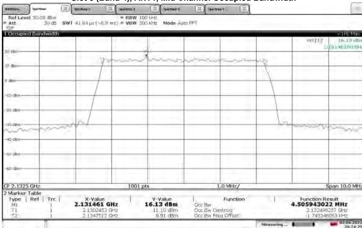
**TM3.1a-256QAM\_5 MHz Bandwidth**
