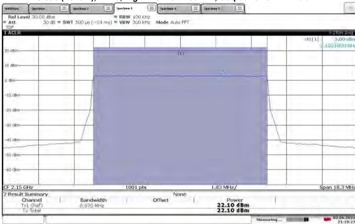
**TM3.1a-256QAM\_10 MHz Bandwidth**
