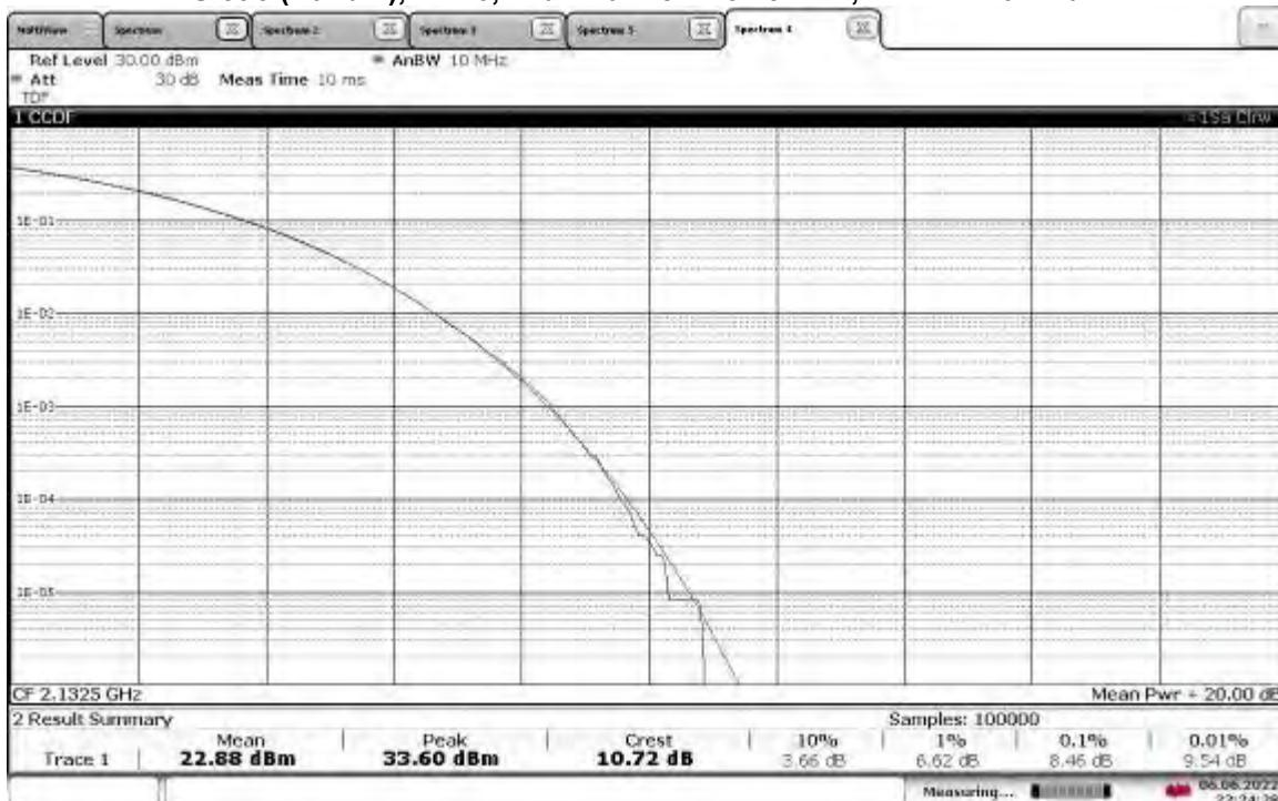
**TM3.1a-256QAM\_10 MHz Bandwidth**
