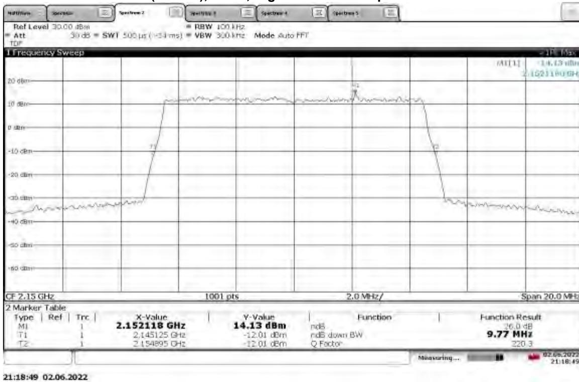
**TM3.1a-256QAM\_10 MHz Bandwidth**
