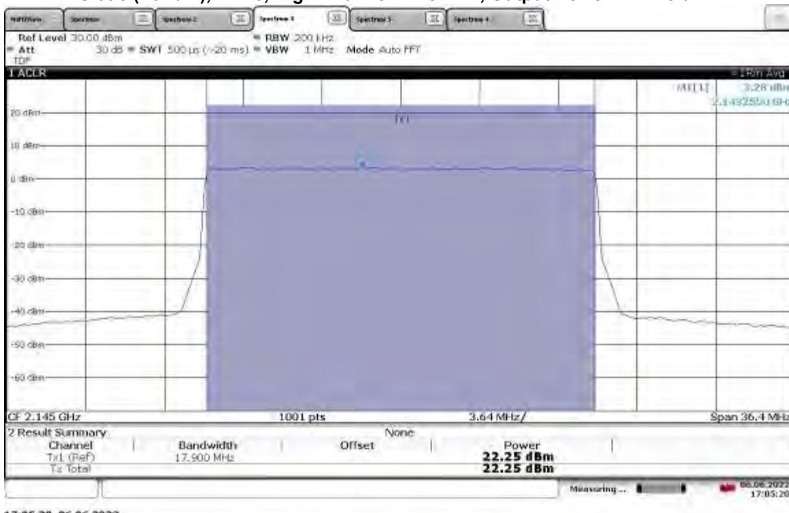
**TM3.1a-256QAM\_20 MHz Bandwidth**
