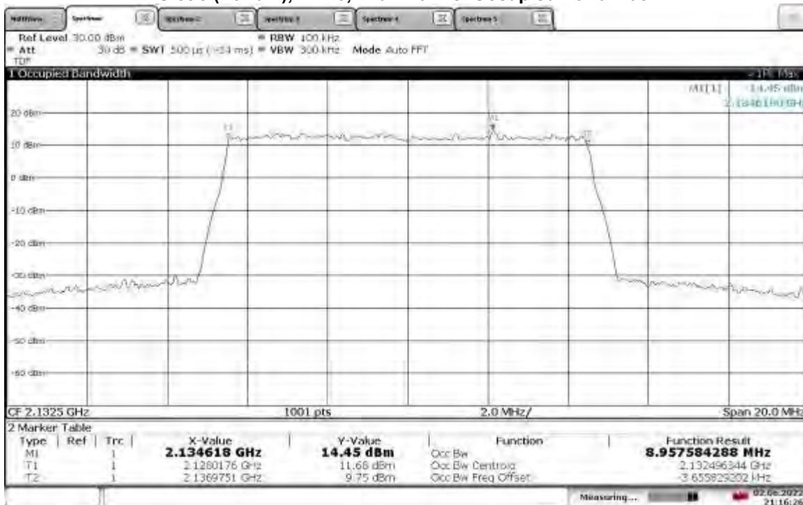
**TM3.1a-256QAM\_10 MHz Bandwidth
