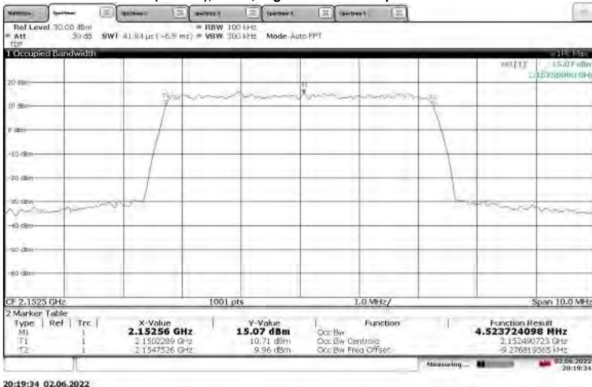
**TM3.1a-256QAM\_5 MHz Bandwidth**
