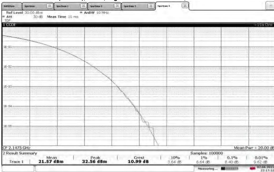
**TM3.1a-256QAM\_15 MHz Bandwidth**
