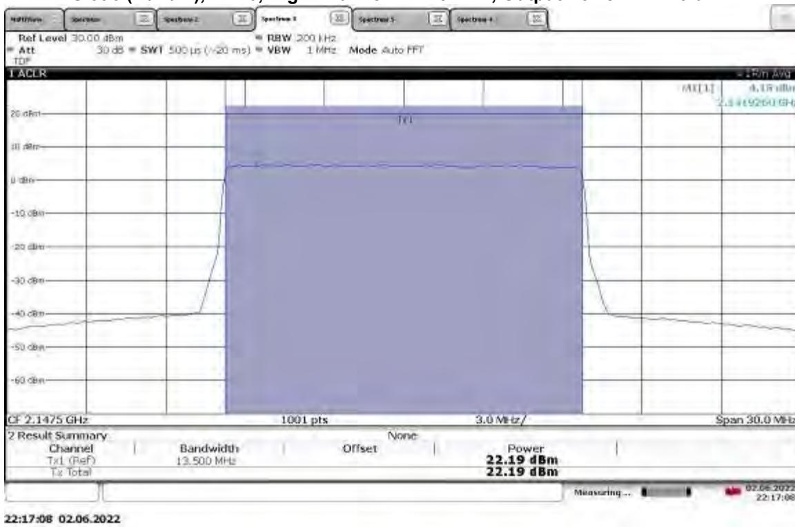
**TM3.1a-256QAM\_15 MHz Bandwidth**
