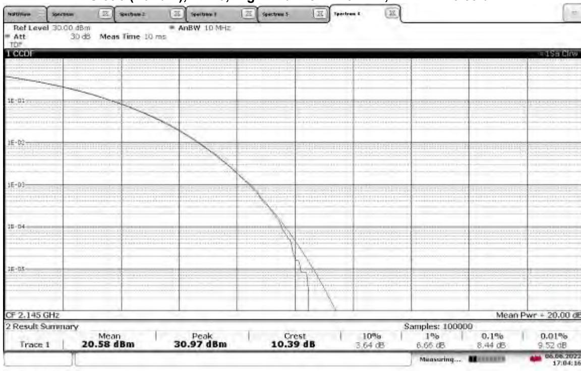
**TM3.1a-256QAM\_20 MHz Bandwidth**
