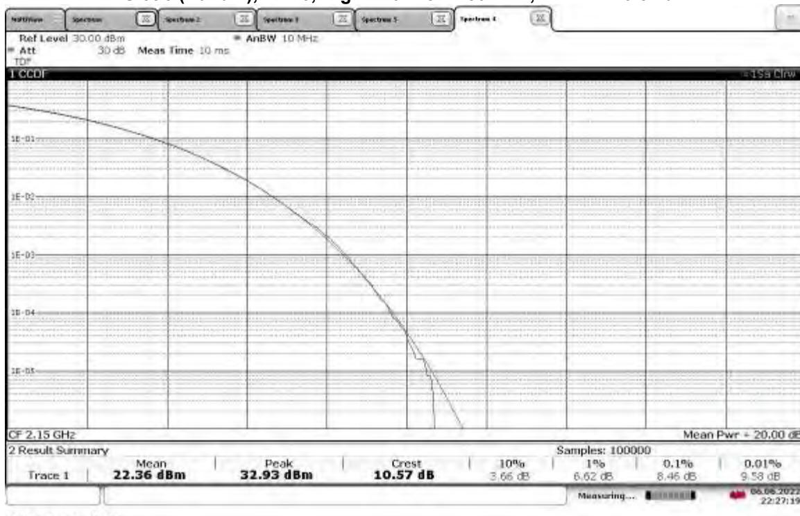
**TM3.1a-256QAM\_10 MHz Bandwidth**
