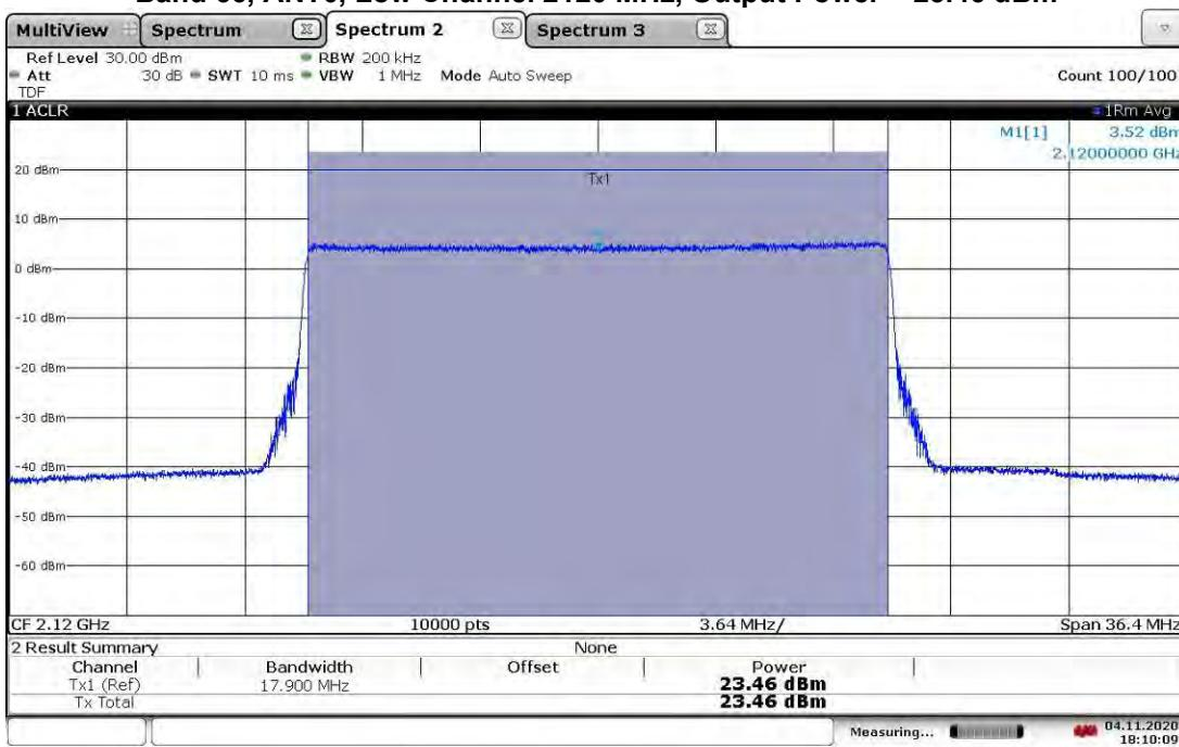
**TM3.1a-256QAM\_20 MHz Bandwidth
