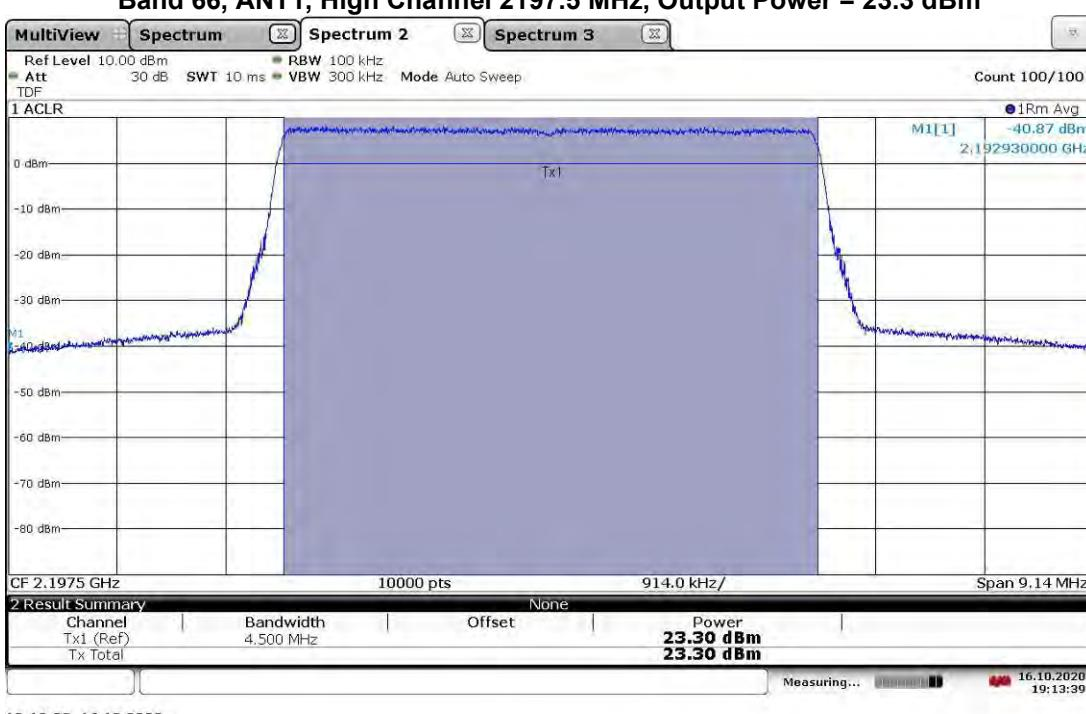
**TM3.1a-256QAM\_10 MHz Bandwidth
