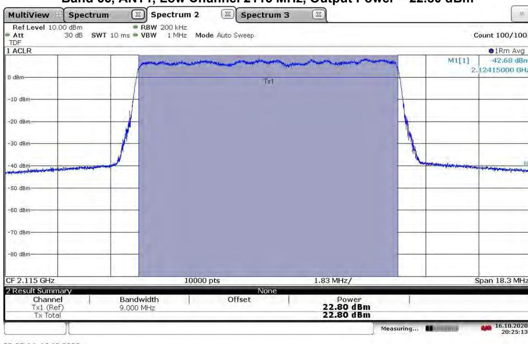
**TM3.1a-256QAM\_10 MHz Bandwidth
