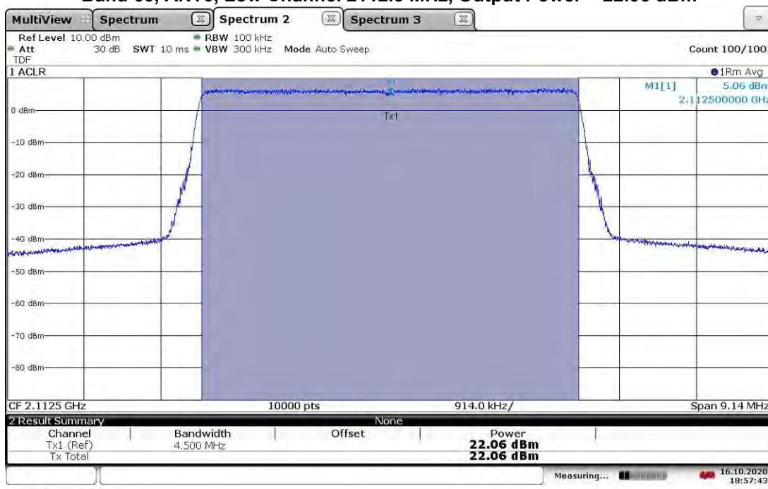
**TM3.1a-256QAM\_5 MHz Bandwidth
