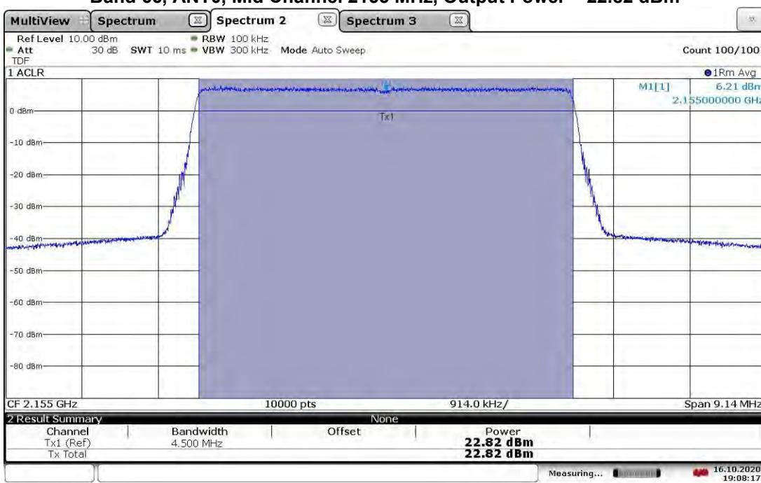
**TM3.1a-256QAM\_5 MHz Bandwidth
