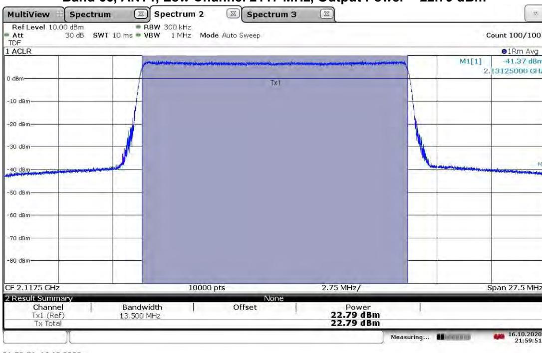
**TM3.1a-256QAM\_15 MHz Bandwidth
