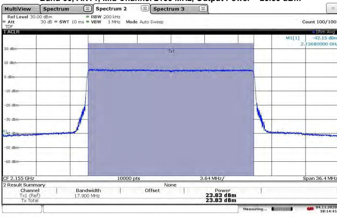
**TM3.1a-256QAM\_20 MHz Bandwidth
