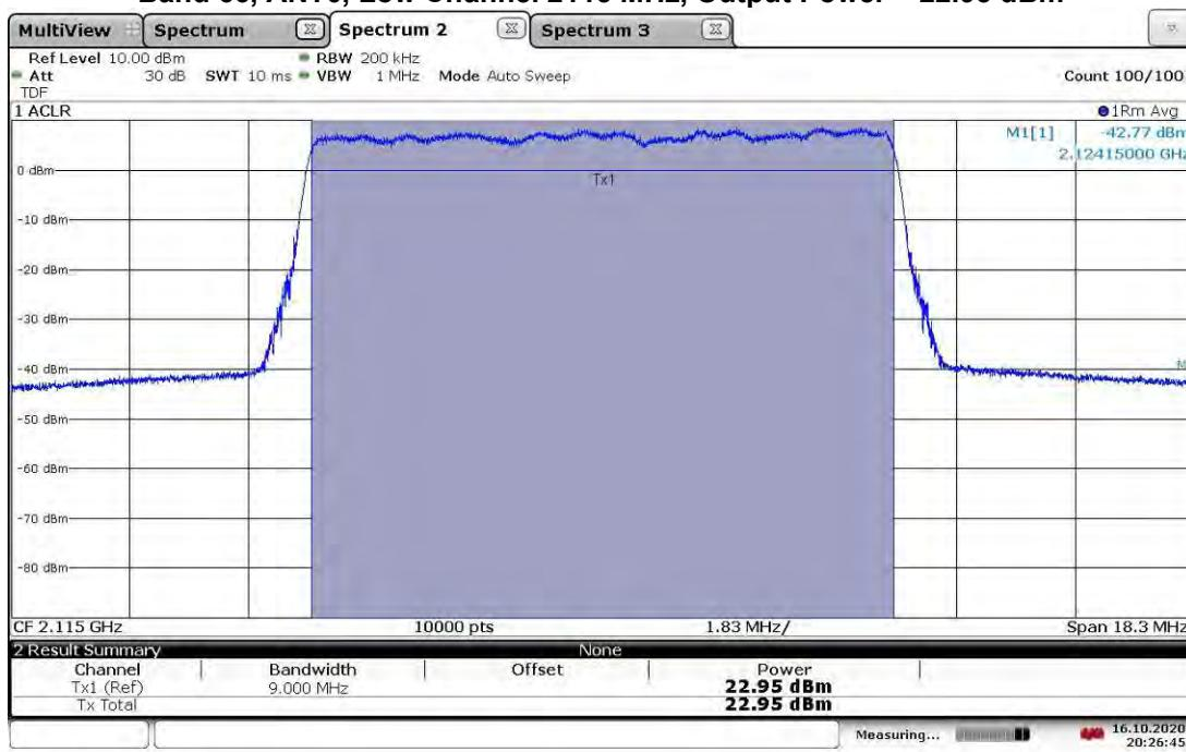
**TM3.1a-256QAM\_10 MHz Bandwidth
