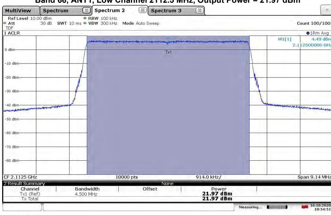
**TM3.1a-256QAM\_5 MHz Bandwidth
