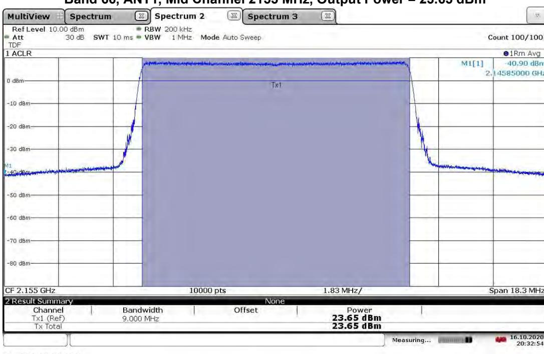
**TM3.1a-256QAM\_10 MHz Bandwidth
