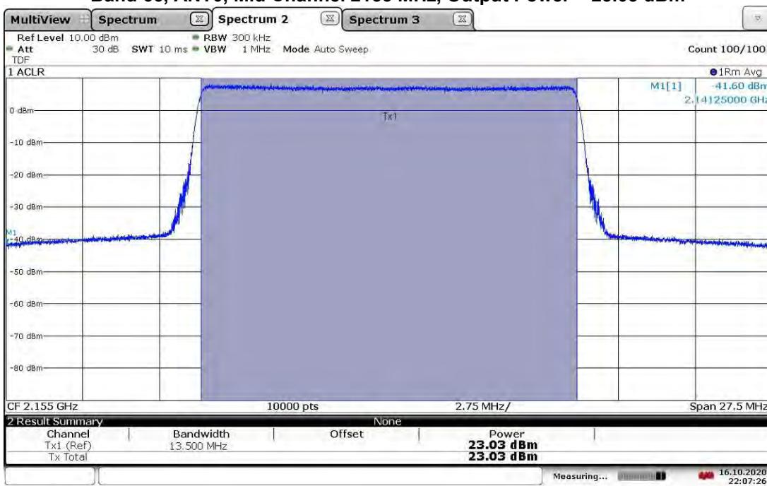
**TM3.1a-256QAM\_15 MHz Bandwidth
