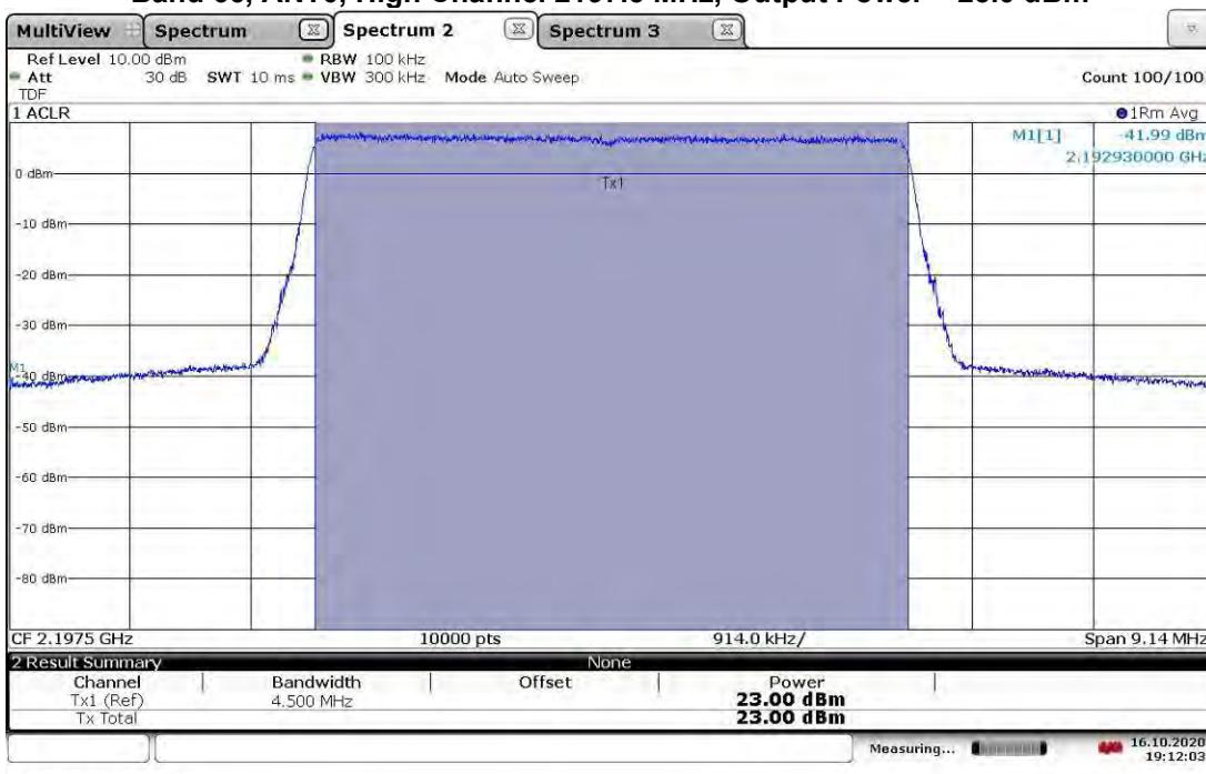
**TM3.1a-256QAM\_5 MHz Bandwidth
