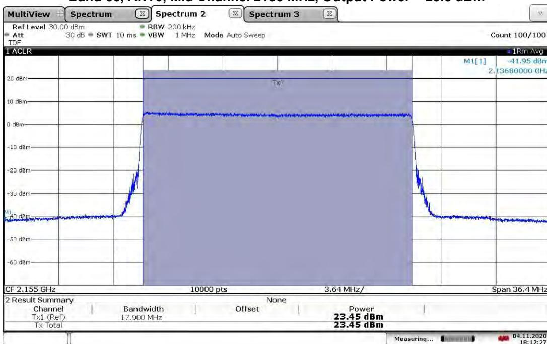
**TM3.1a-256QAM\_20 MHz Bandwidth
