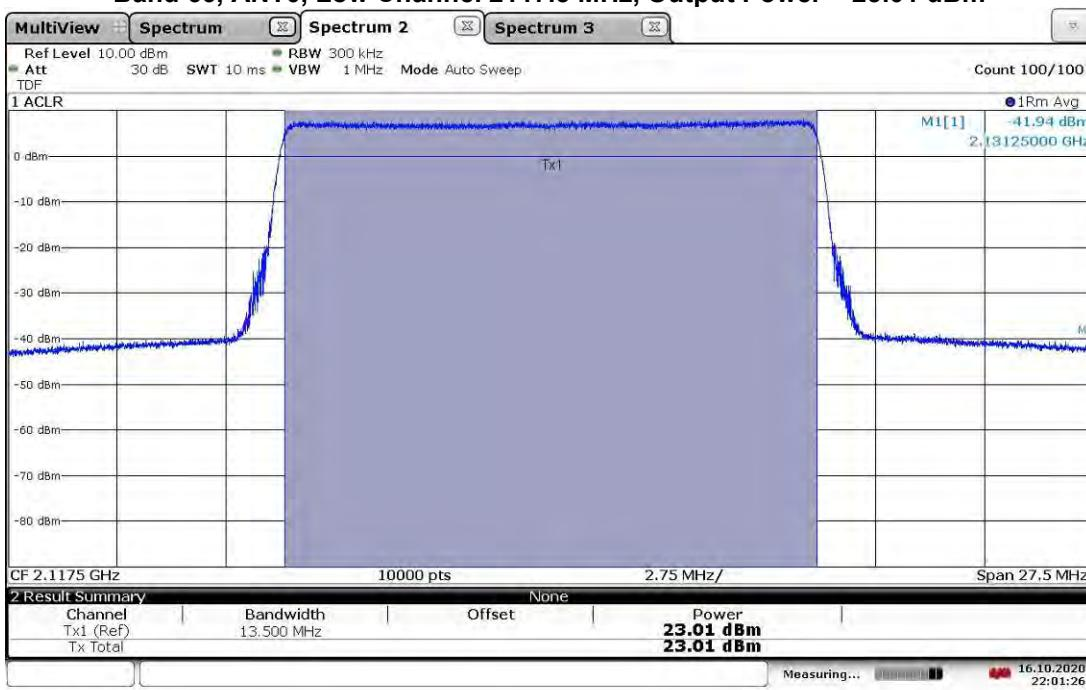
**TM3.1a-256QAM\_15 MHz Bandwidth
