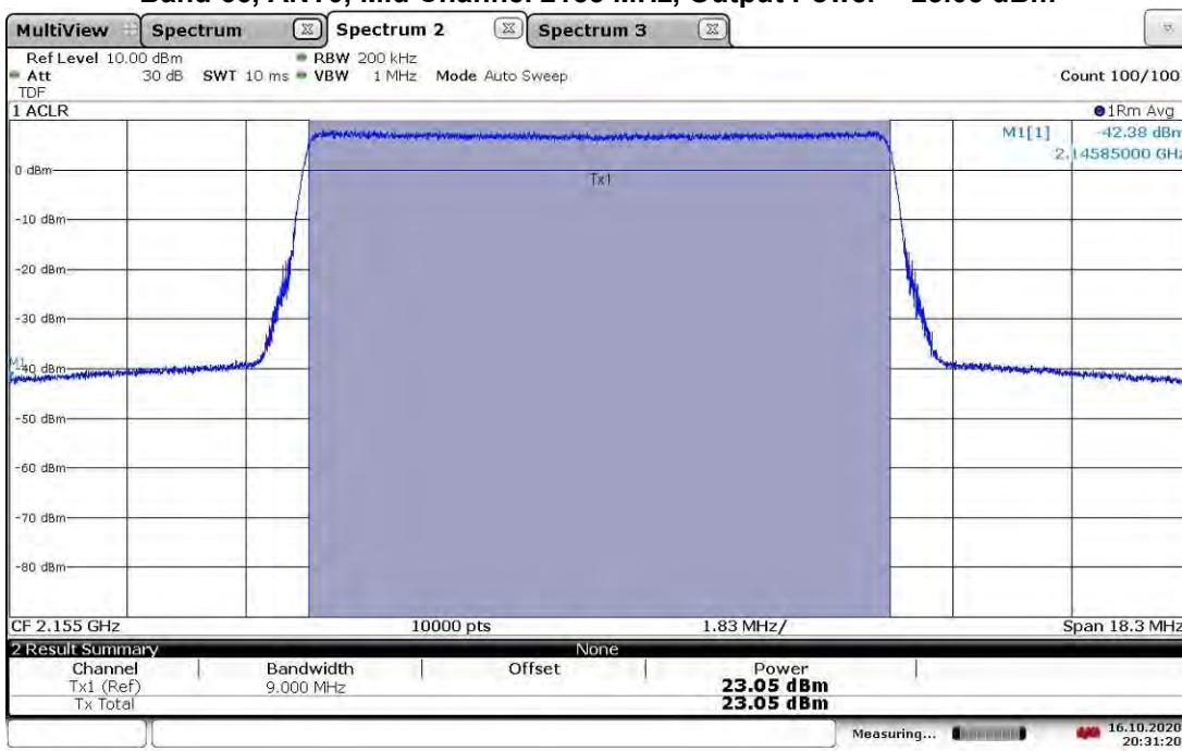
**TM3.1a-256QAM\_10 MHz Bandwidth
