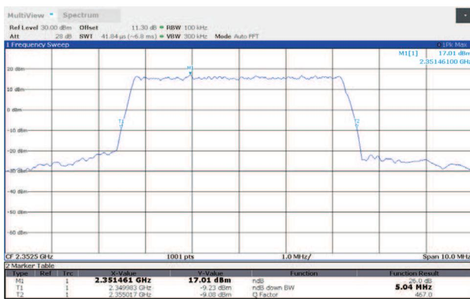
**TM3.1a-256QAM\_5 MHz Bandwidth
