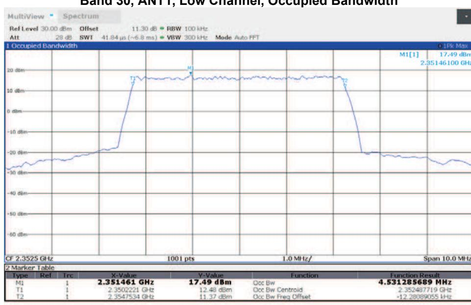
**TM3.1a-256QAM\_5 MHz Bandwidth
