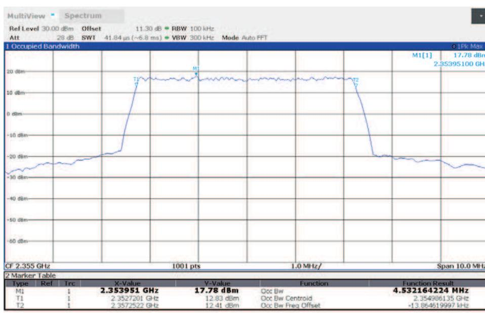
**TM3.1a-256QAM\_5 MHz Bandwidth
