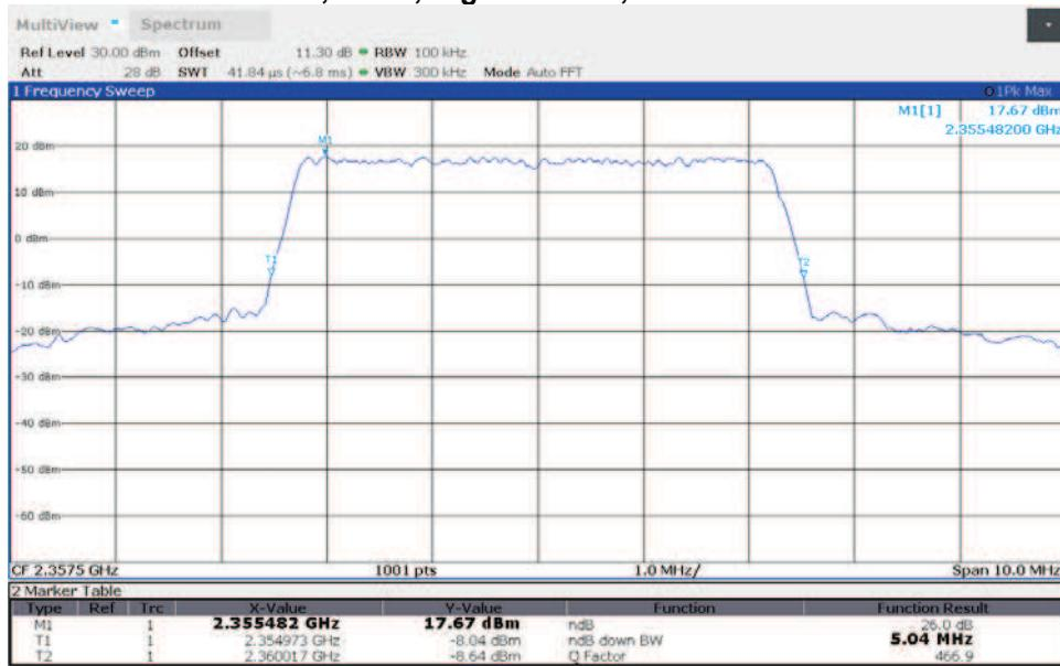
**TM3.1a-256QAM\_5 MHz Bandwidth
