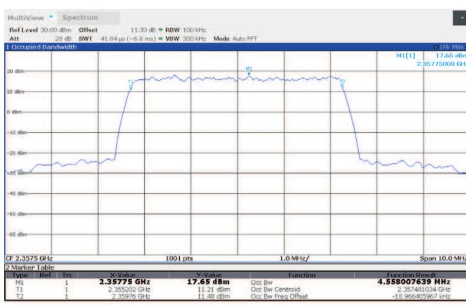
**TM3.1a-256QAM\_5 MHz Bandwidth
