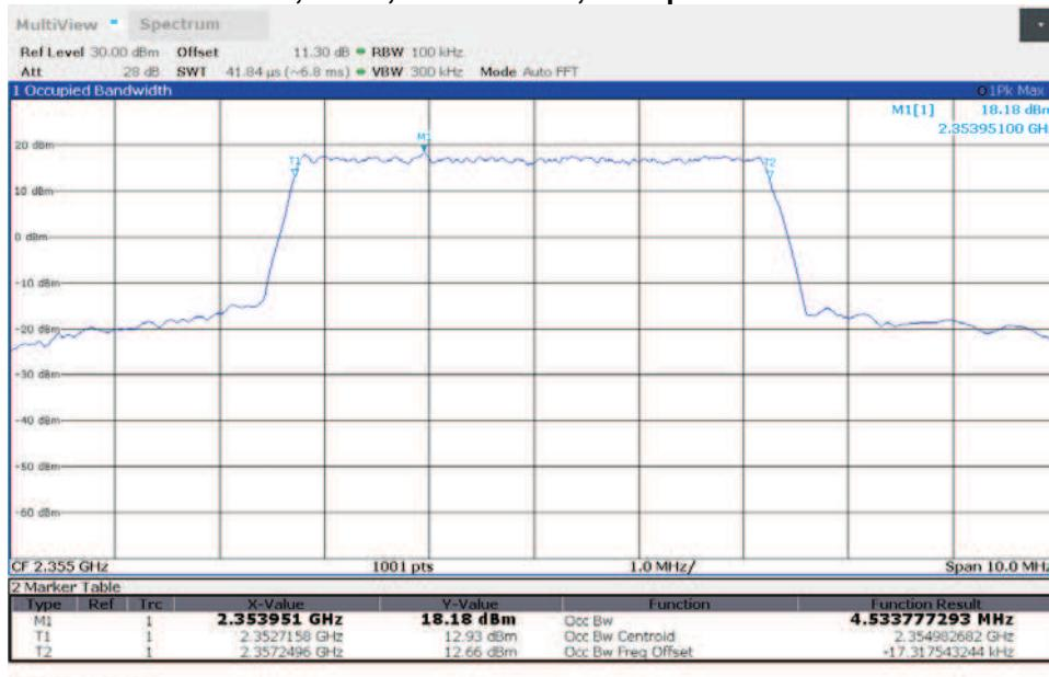
**TM3.1a-256QAM\_5 MHz Bandwidth
