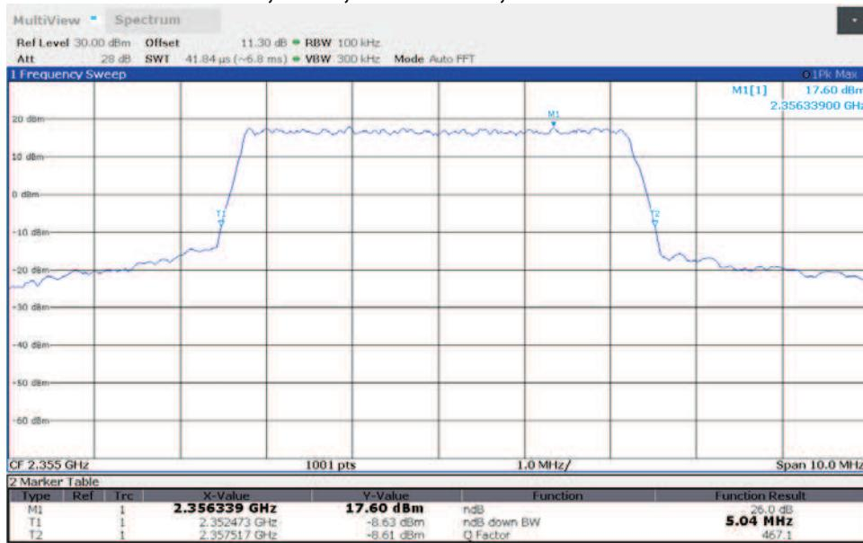
**TM3.1a-256QAM\_5 MHz Bandwidth
