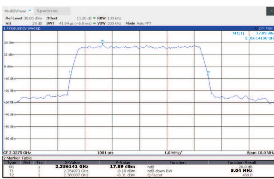
**TM3.1a-256QAM\_5 MHz Bandwidth
