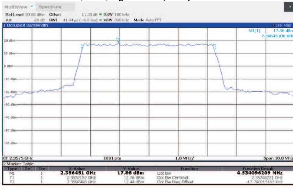
**TM3.1a-256QAM\_5 MHz Bandwidth
