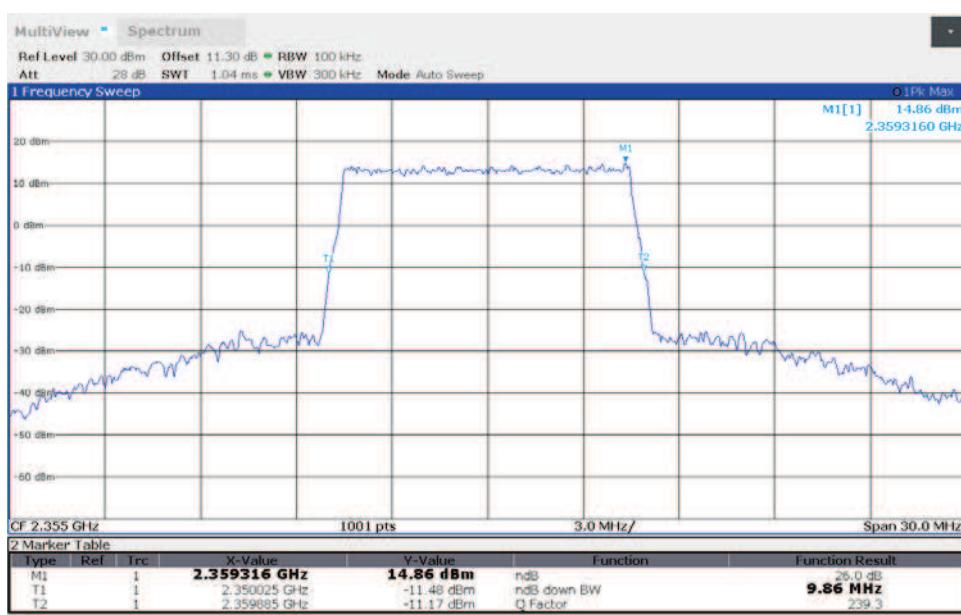
**TM3.1a-256QAM\_10 MHz Bandwidth
