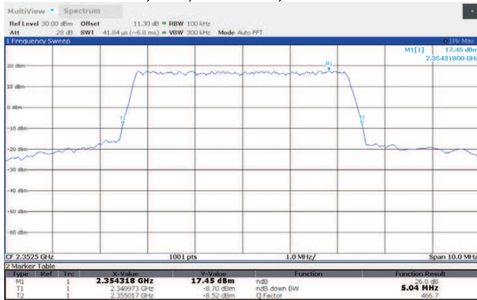
**TM3.1a-256QAM\_5 MHz Bandwidth
