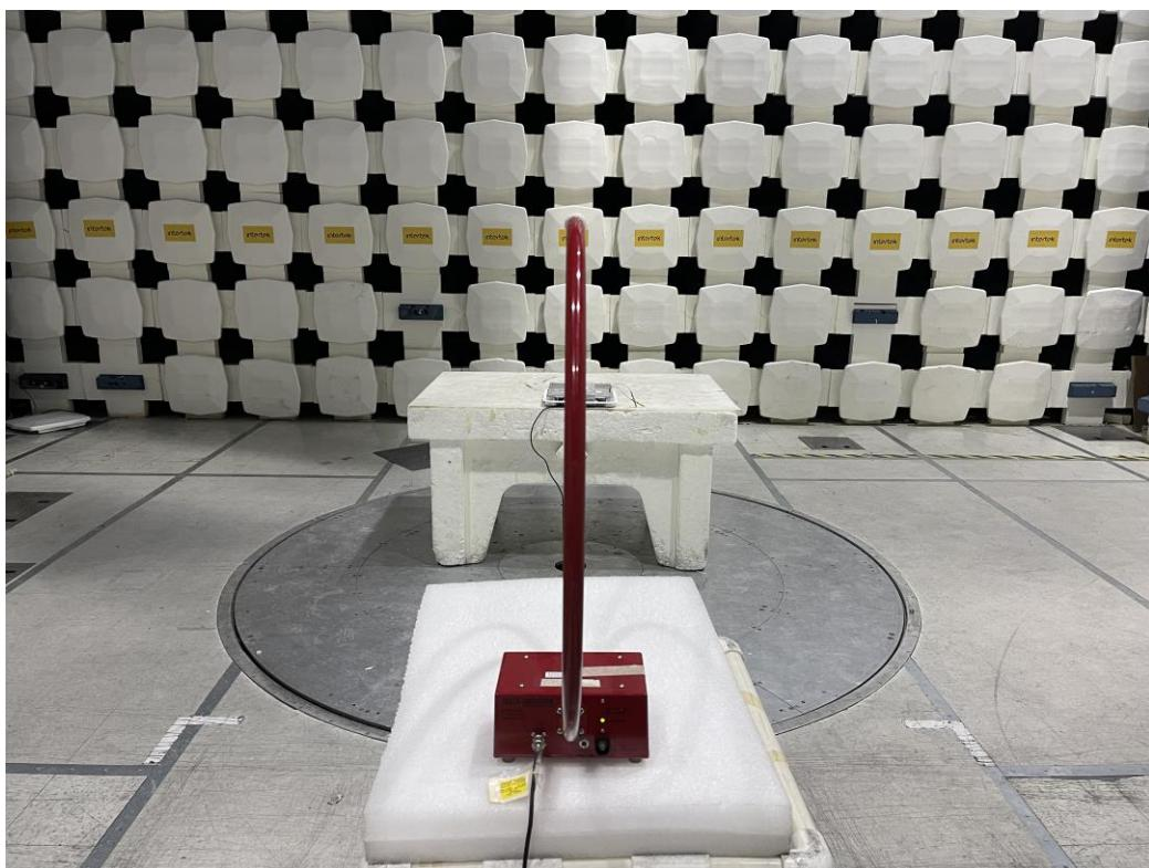
9 kHz-30 MHz Radiated Emissions Test Setup
