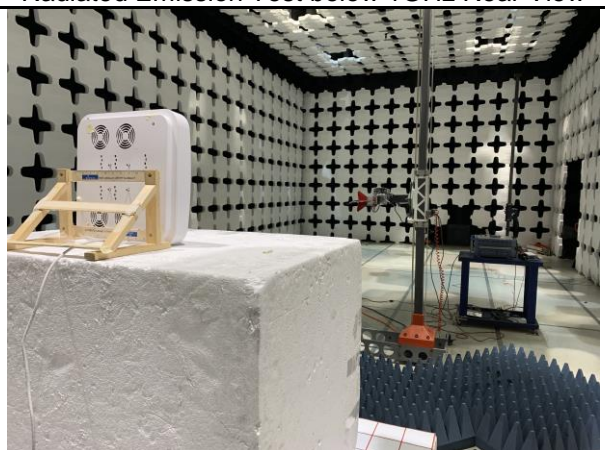
Radiated Emission Test Above 1GHz Rear View
