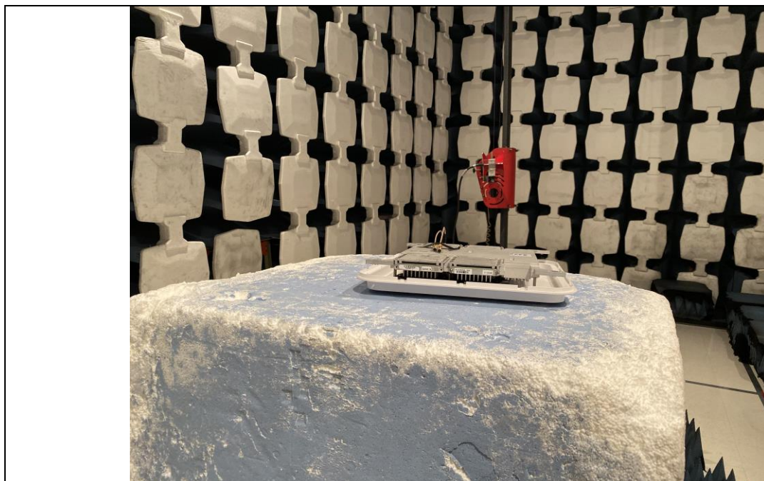
Radiated Emission Test above 1GHz Front View
