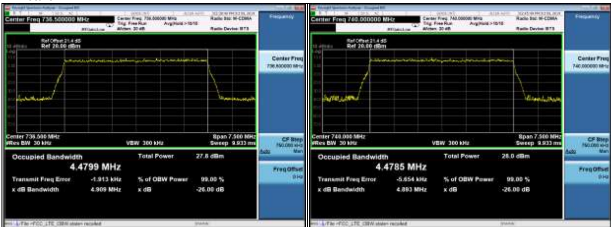
5MHz, QPSK, Low Channel
