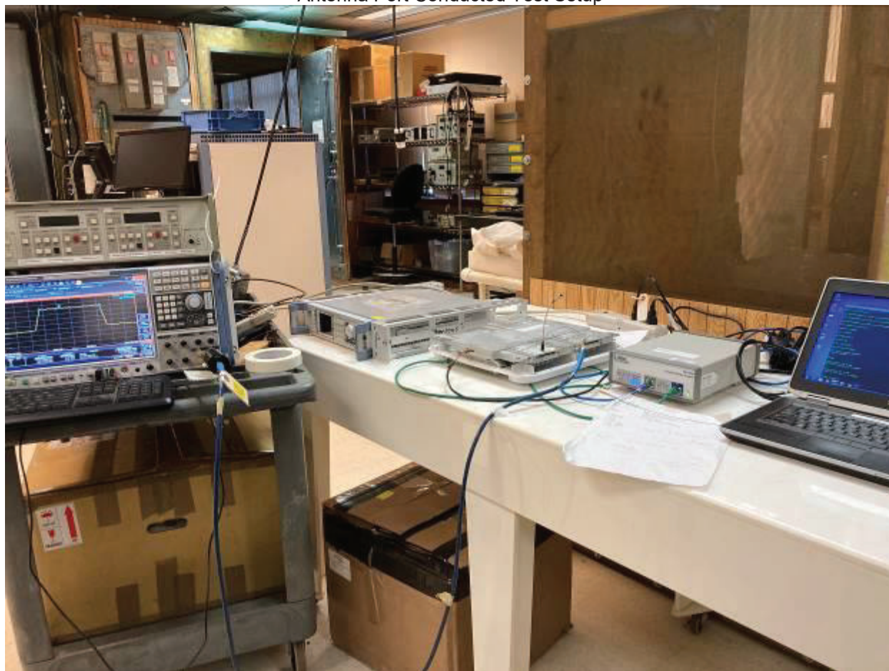
Antenna Port Conducted Test Setup
