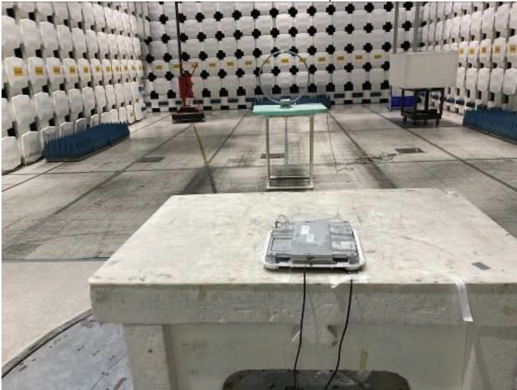
9kHz-30 MHz Test Setup
