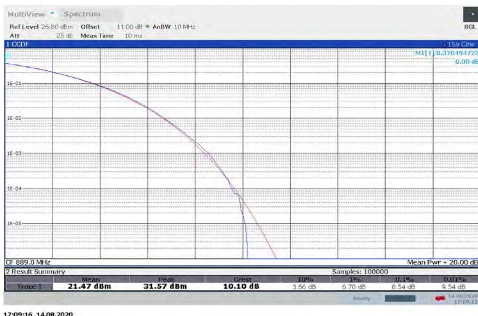
**TM3.1a-256QAM\_10 MHz Bandwidth
