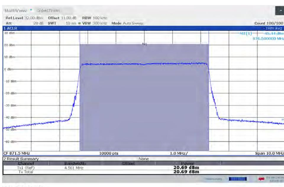
**TM3.1a-256QAM\_5 MHz Bandwidth
