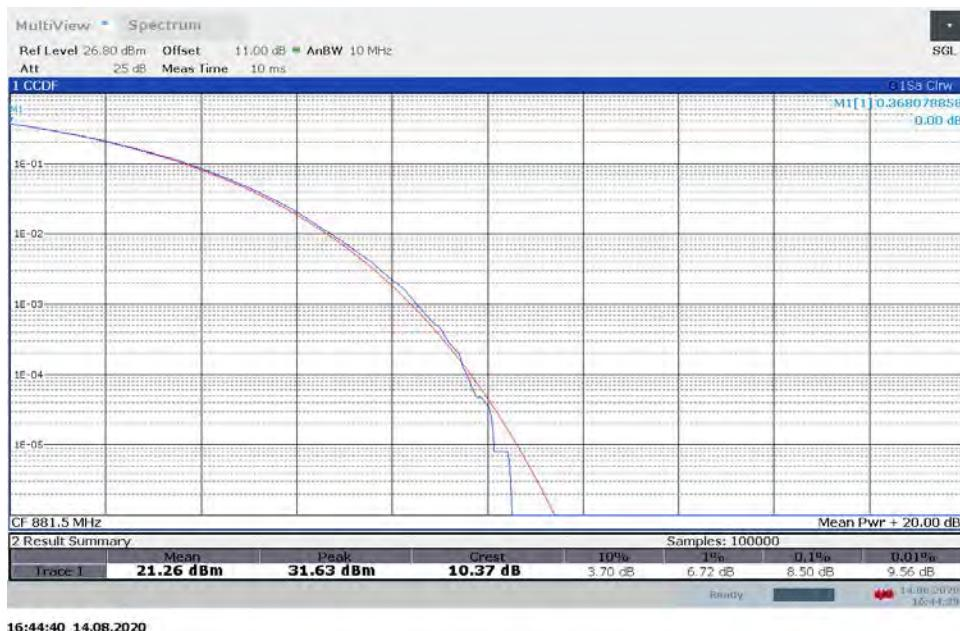
**TM3.1a-256QAM\_5 MHz Bandwidth
