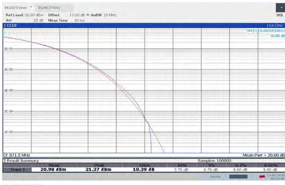
**TM3.1a-256QAM\_5 MHz Bandwidth
