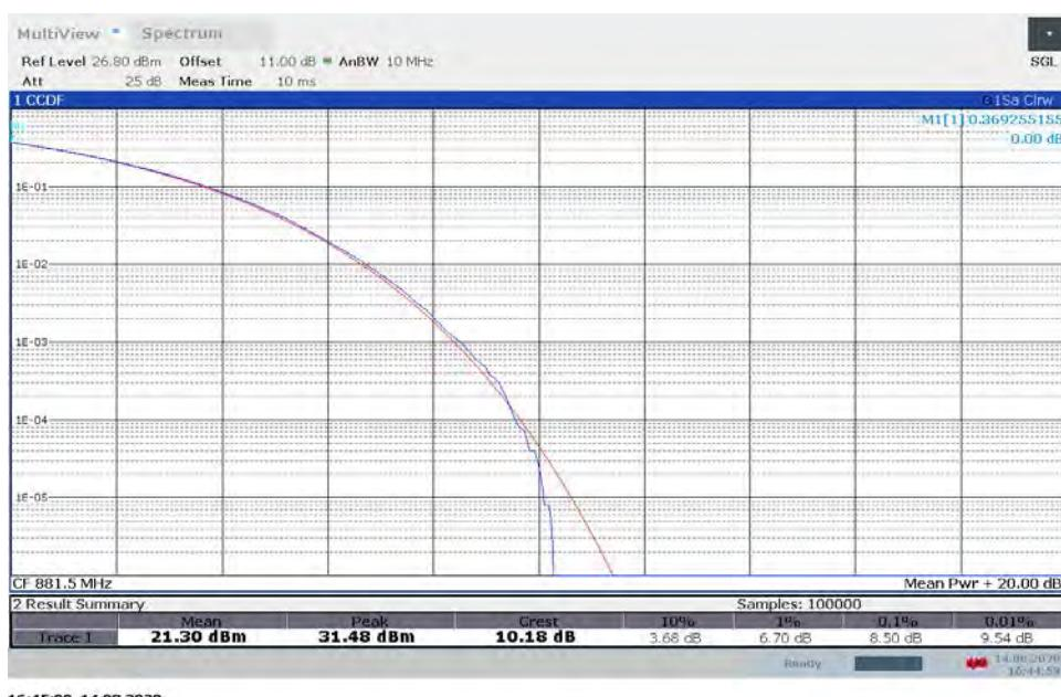
**TM3.1a-256QAM\_5 MHz Bandwidth
