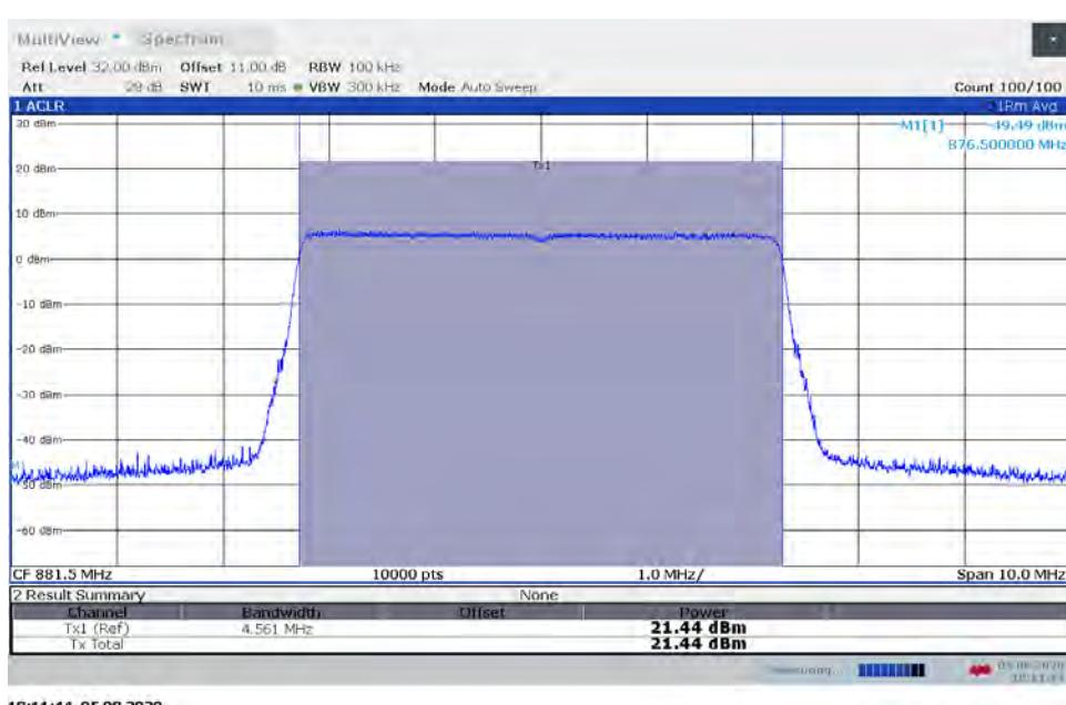
**TM3.1a-256QAM\_5 MHz Bandwidth
