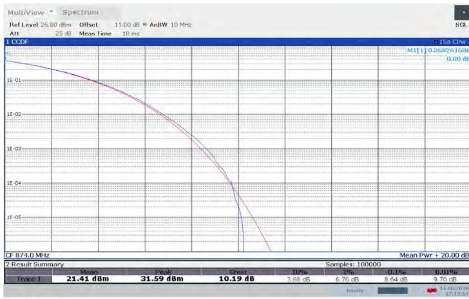
**TM3.1a-256QAM\_10 MHz Bandwidth
