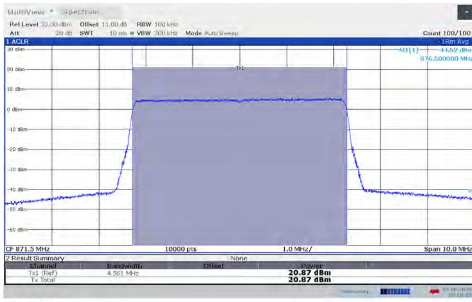
**TM3.1a-256QAM\_5 MHz Bandwidth
