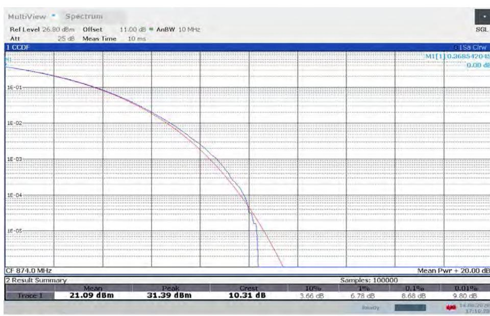
**TM3.1a-256QAM\_10 MHz Bandwidth
