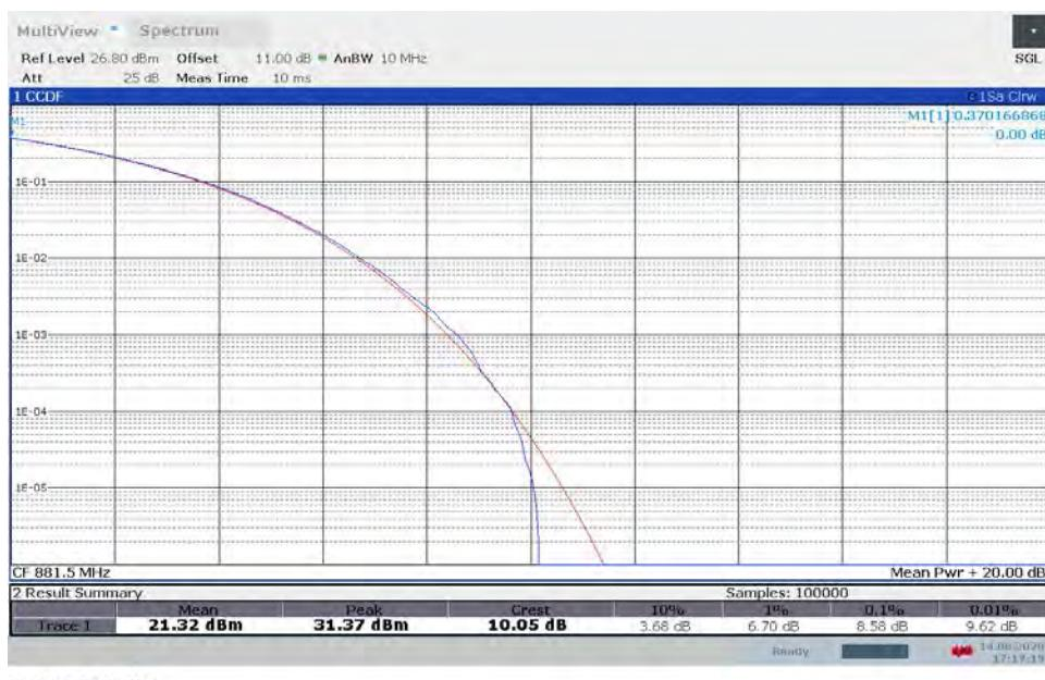
**TM3.1a-256QAM\_10 MHz Bandwidth
