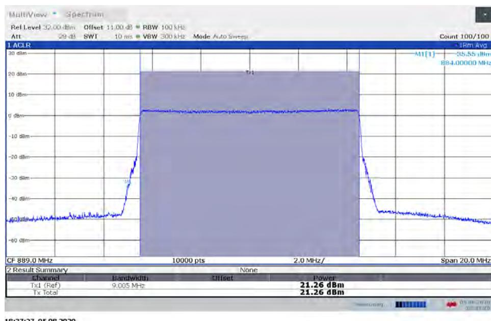
**TM3.1a-256QAM\_10 MHz Bandwidth
