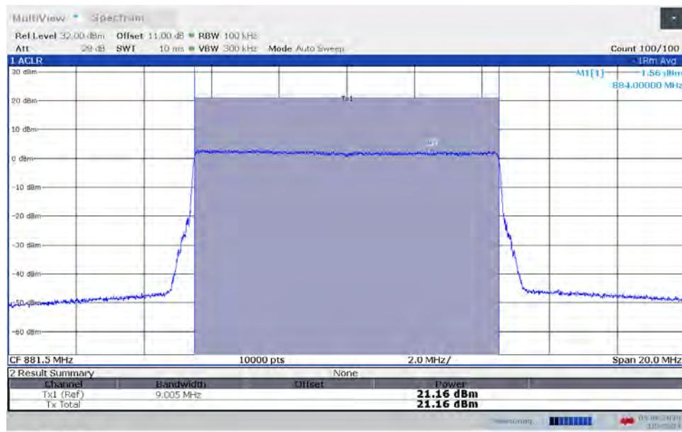
**TM3.1a-256QAM\_10 MHz Bandwidth
