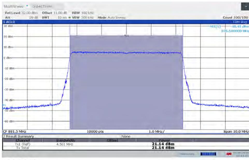
**TM3.1a-256QAM\_5 MHz Bandwidth
