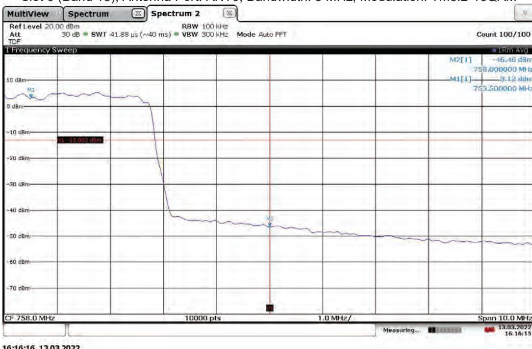
Band Edge Compliant, Upper Band Edge, 753.5MHz (4G LTE) With RP5200 Host Slot 0 (Band 13), Antenna Port: ANT1, Bandwidth: 5 MHz, Modulation: TM3.2-16QAM
