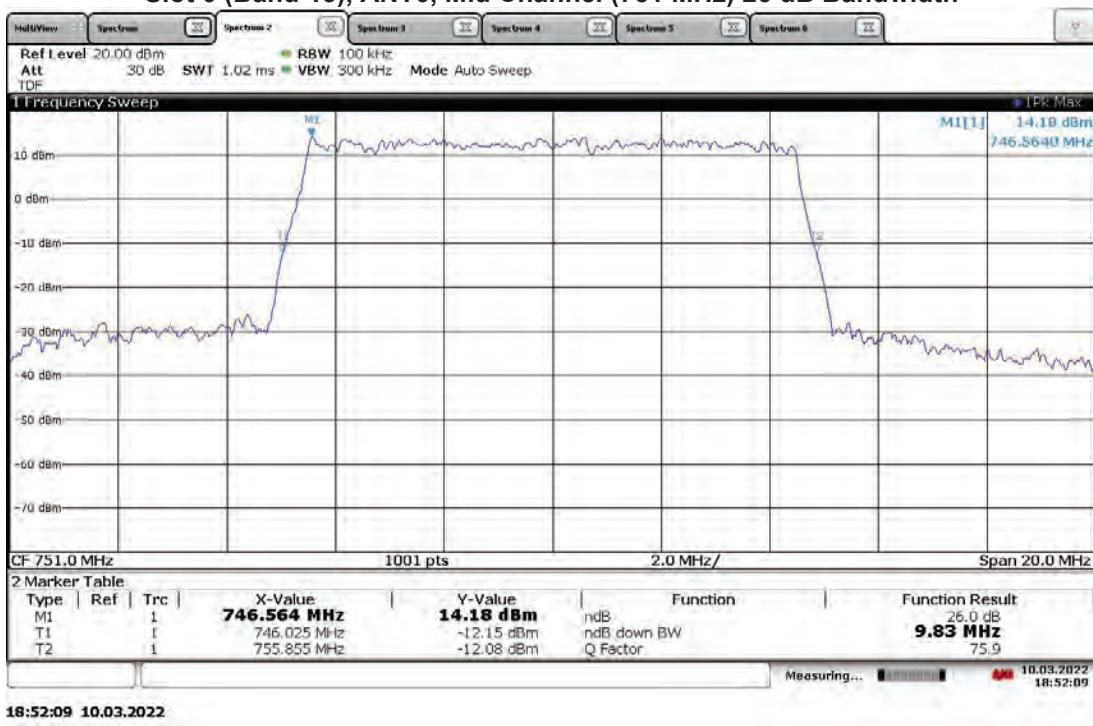
**TM3.2-16QAM\_10 MHz Bandwidth (4G LTE) With RP5200 Host
