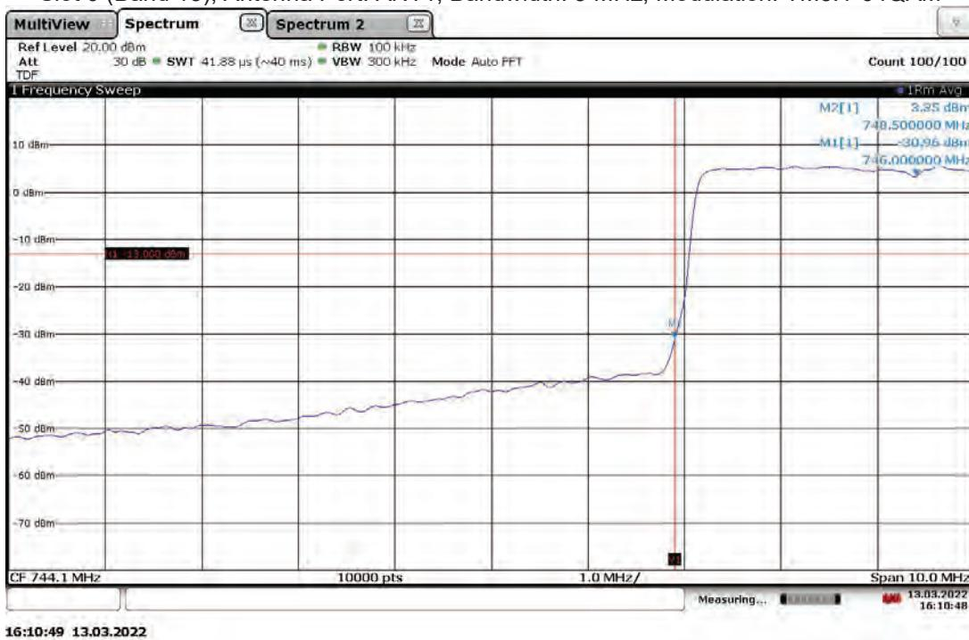
Band Edge Compliant, Upper Band Edge, 753.5 MHz (4G LTE) With RP5200 Host Slot 0 (Band 13), Antenna Port: ANT0, Bandwidth: 5 MHz, Modulation: TM3.1-64QAM
