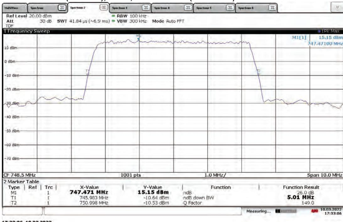
**TM3.1-64QAM\_5 MHz Bandwidth (4G LTE) With RP5200 Host
