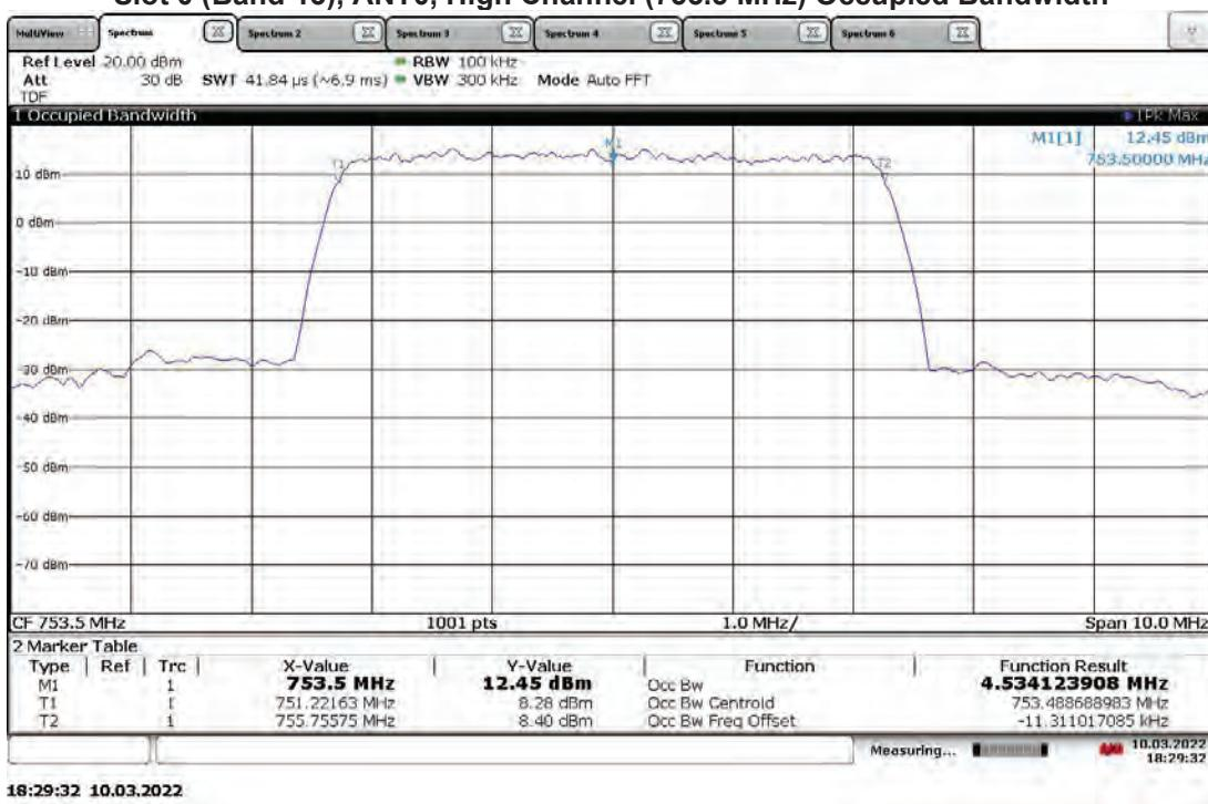
**TM3.1-64QAM\_5 MHz Bandwidth (4G LTE) With RP5200 Host
