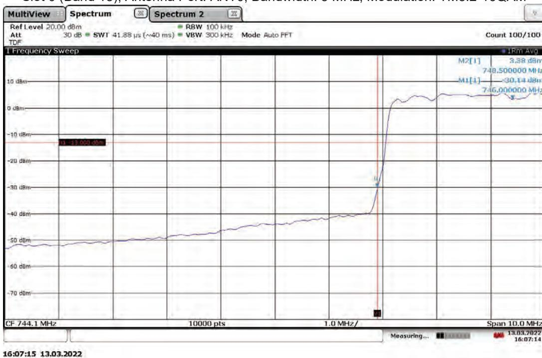
Band Edge Compliant, Lower Band Edge, 748.5 MHz (4G LTE) With RP5200 Host Slot 0 (Band 13), Antenna Port: ANT1, Bandwidth: 5 MHz, Modulation: TM3.2-16QAM
