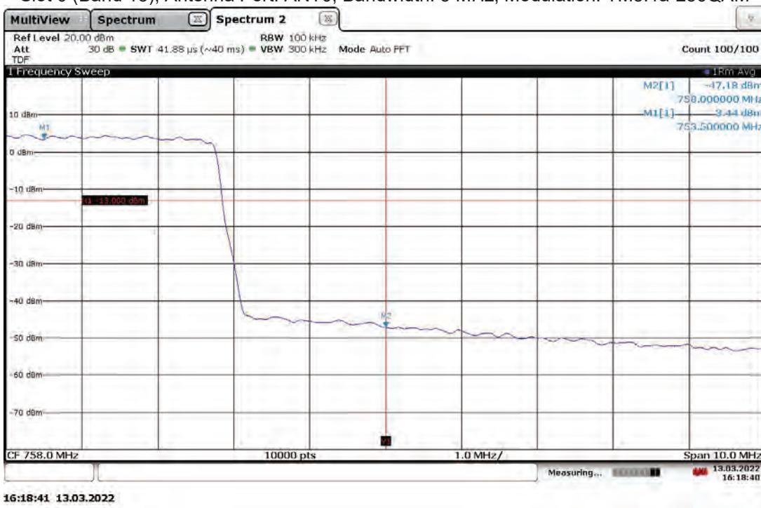
Band Edge Compliant, Upper Band Edge, 753.5 MHz (4G LTE) With RP5200 Host Slot 0 (Band 13), Antenna Port: ANT1, Bandwidth: 5 MHz, Modulation: TM3.1a-256QAM
