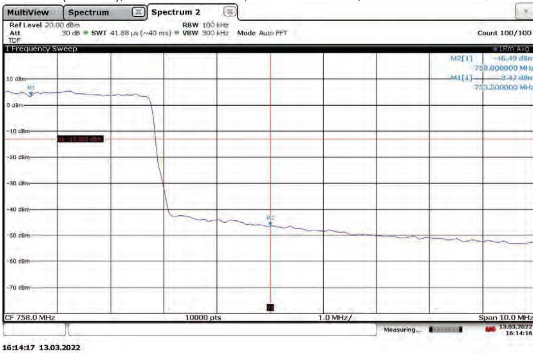
Band Edge Compliant, Lower Band Edge, 748.5 MHz (4G LTE) With RP5200 Host Slot 0 (Band 13), Antenna Port: ANT0, Bandwidth: 5 MHz, Modulation: TM3.2-16QAM
