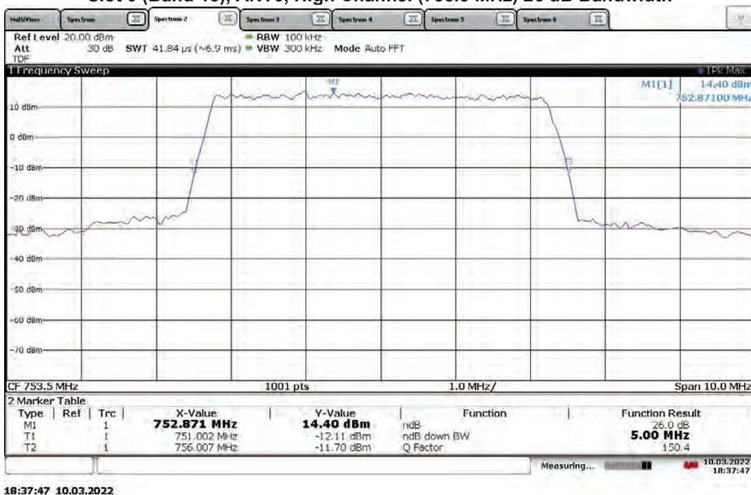
**TM3.1a-256QAM\_5 MHz Bandwidth (4G LTE) With RP5200 Host
