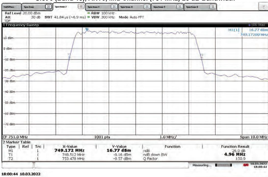
**TM3.2-16QAM\_5 MHz Bandwidth (4G LTE) With RP5200 Host
