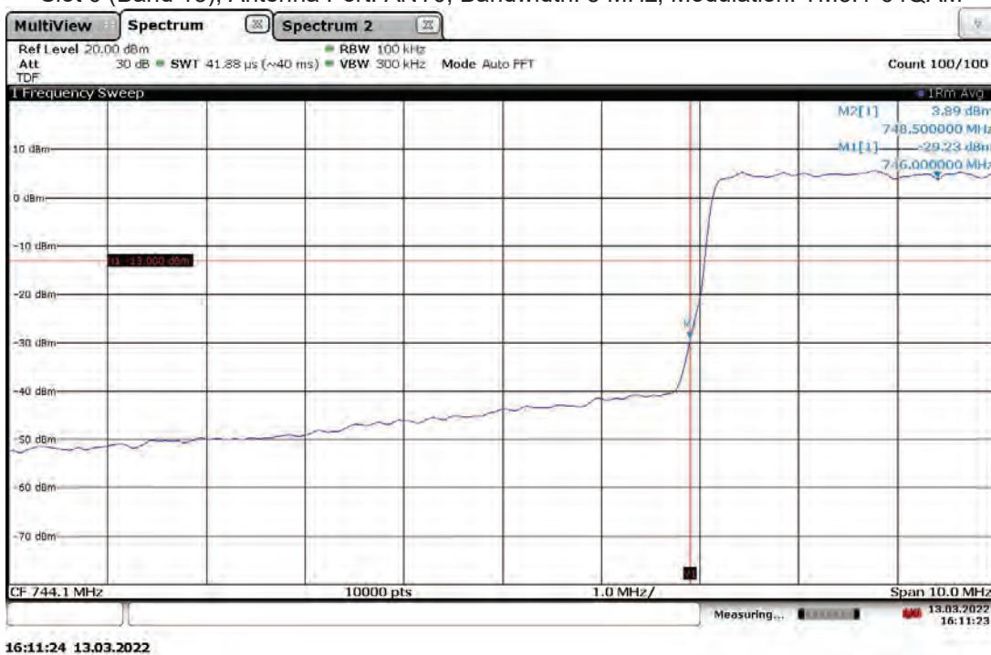
Band Edge Compliant, Lower Band Edge, 748.5 MHz (4G LTE) With RP5200 Host Slot 0 (Band 13), Antenna Port: ANT1, Bandwidth: 5 MHz, Modulation: TM3.1-64QAM
