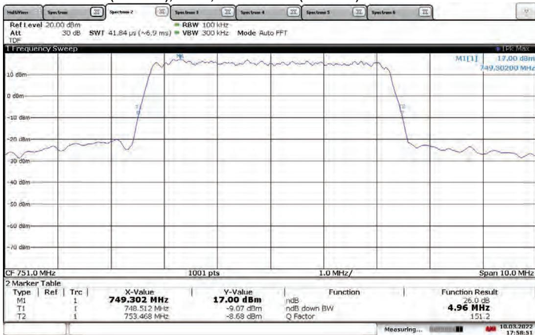
**TM3.2-16QAM\_5 MHz Bandwidth (4G LTE) With RP5200 Host
