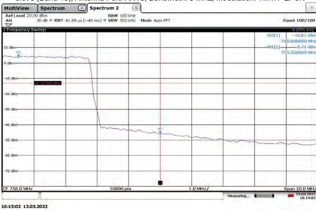
Band Edge Compliant, Upper Band Edge, 753.5 MHz (4G LTE) With RP5200 Host Slot 0 (Band 13), Antenna Port: ANT1, Bandwidth: 5 MHz, Modulation: TM1.1-QPSK
