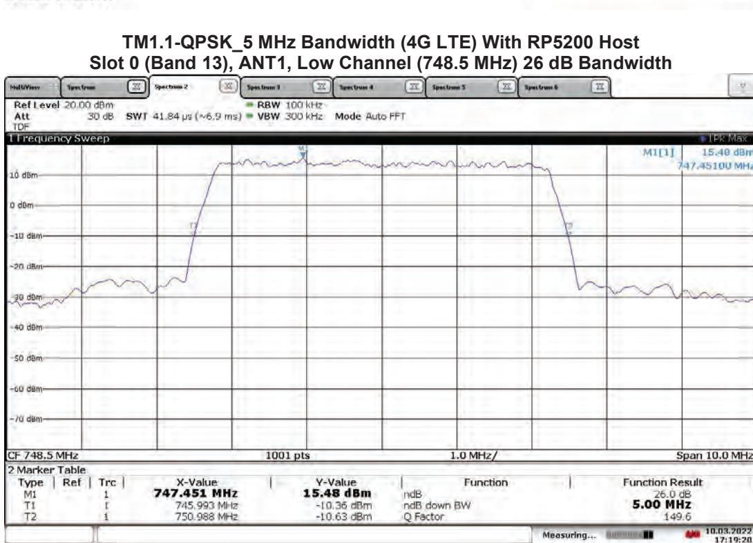
**TM1.1-QPSK\_5 MHz Bandwidth (4G LTE) With RP5200 Host
