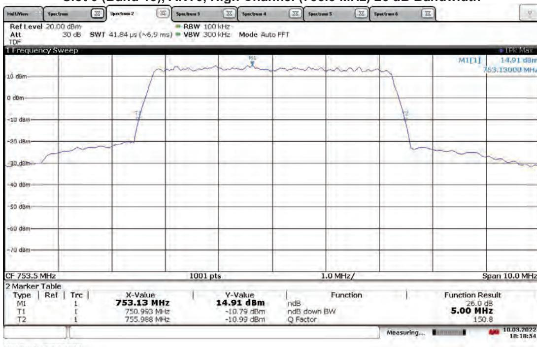
**TM1.1-QPSK\_5 MHz Bandwidth (4G LTE) With RP5200 Host
