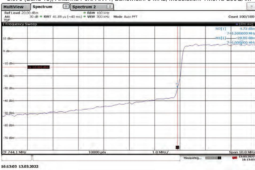
Band Edge Compliant, Upper Band Edge, 753.5 MHz (4G LTE) With RP5200 Host Slot 0 (Band 13), Antenna Port: ANT0, Bandwidth: 5 MHz, Modulation: TM3.1a-256QAM
