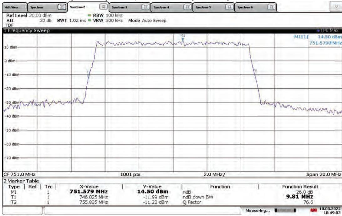
**TM3.1-64QAM\_10 MHz Bandwidth (4G LTE) With RP5200 Host
