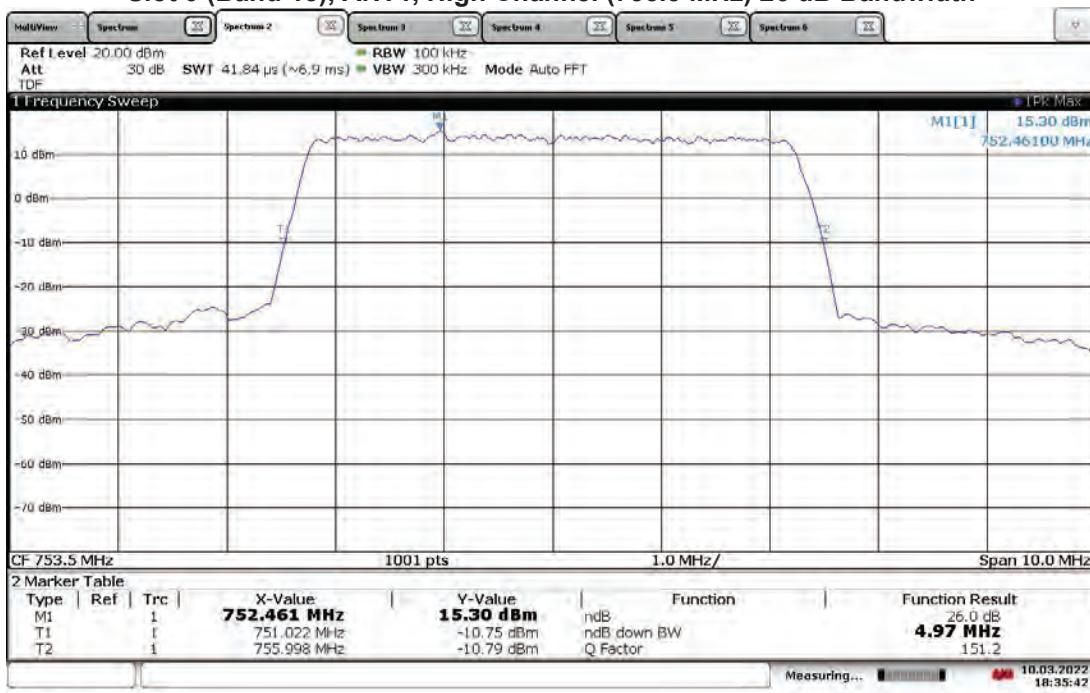
**TM1.1-QPSK\_10 MHz Bandwidth (4G LTE) With RP5200 Host
