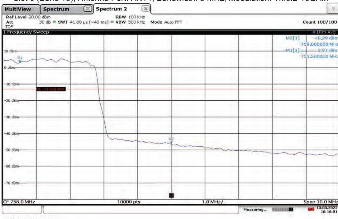
Band Edge Compliant, Lower Band Edge, 748.5 MHz (4G LTE) With RP5200 Host Slot 0 (Band 13), Antenna Port: ANT0, Bandwidth: 5 MHz, Modulation: TM3.1-64QAM
