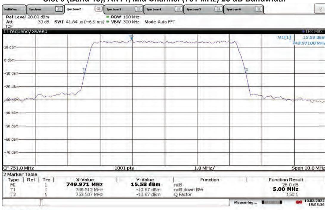
**TM3.1a-256QAM\_5 MHz Bandwidth (4G LTE) With RP5200 Host
