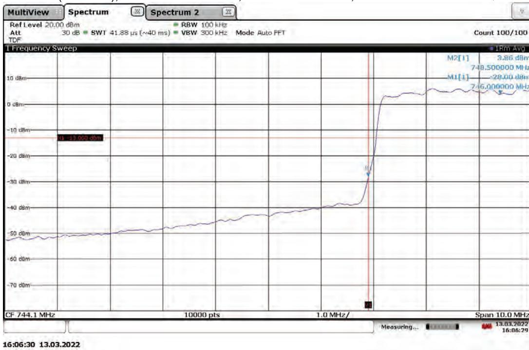
Band Edge Compliant, Upper Band Edge, 753.5MHz (4G LTE) With RP5200 Host Slot 0 (Band 13), Antenna Port: ANT0, Bandwidth: 5 MHz, Modulation: TM3.2-16QAM
