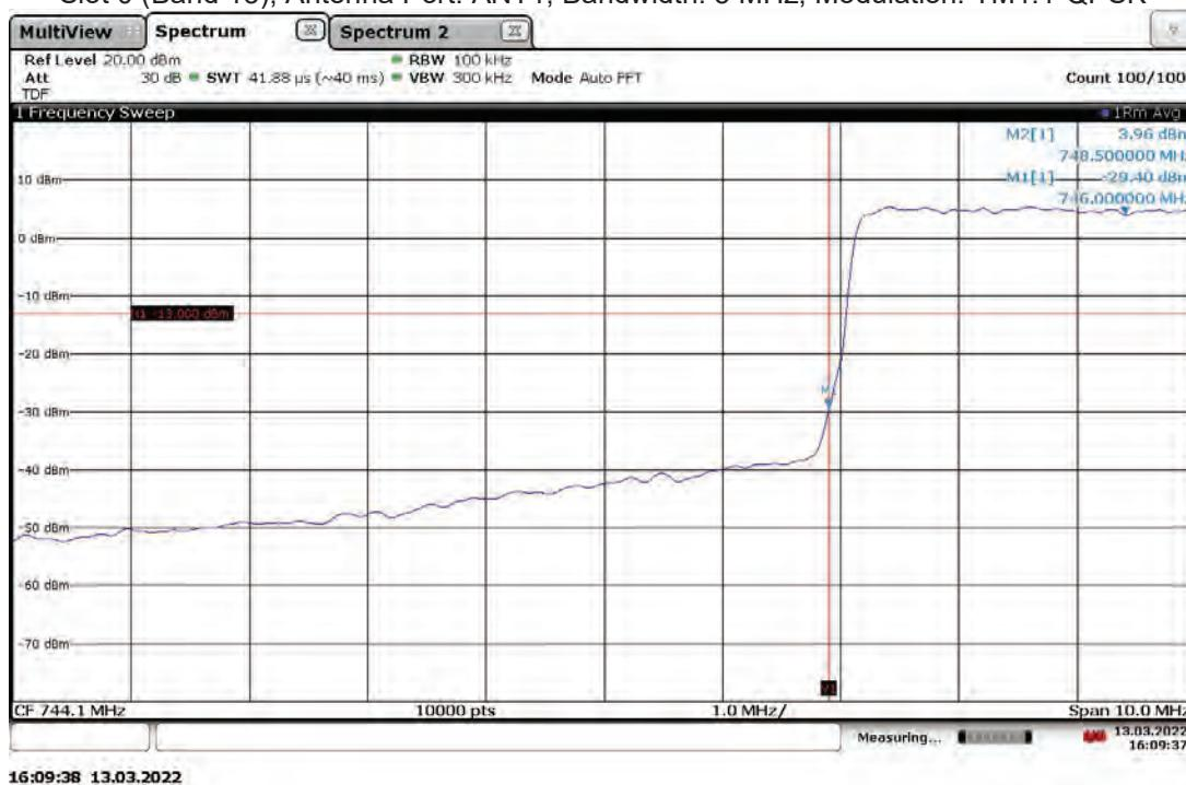
Band Edge Compliant, Upper Band Edge, 753.5 MHz (4G LTE) With RP5200 Host Slot 0 (Band 13), Antenna Port: ANT0, Bandwidth: 5 MHz, Modulation: TM1.1-QPSK
