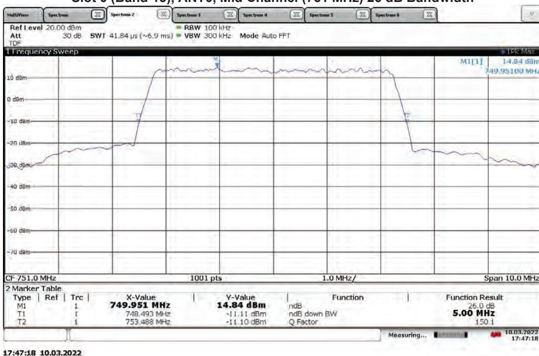
**TM1.1-QPSK\_5 MHz Bandwidth (4G LTE) With RP5200 Host
