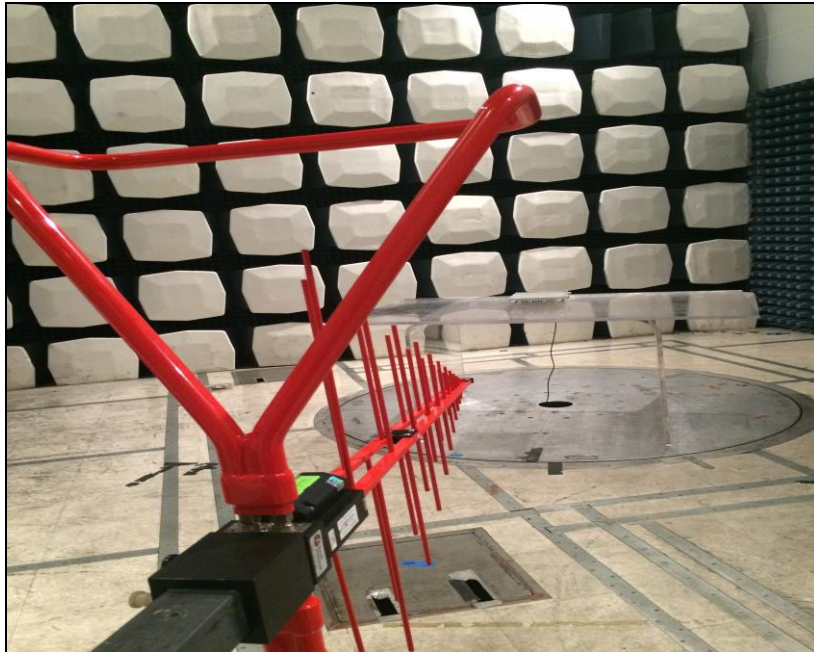
Photograph 1. Radiated Spurious Emissions 30 MHz – 1 GHz, Test Setup
