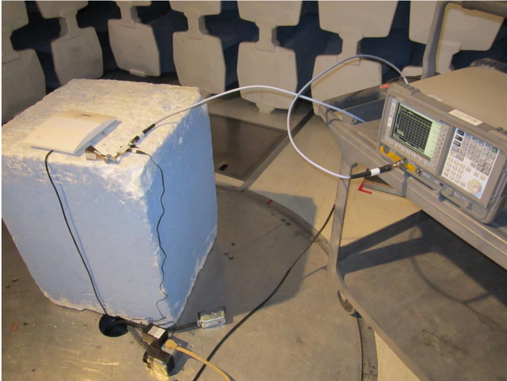
Radiated Spurious EMI – (18 to 22GHz)
