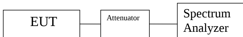
Figure 3. Power Spectral Density Test Setup
