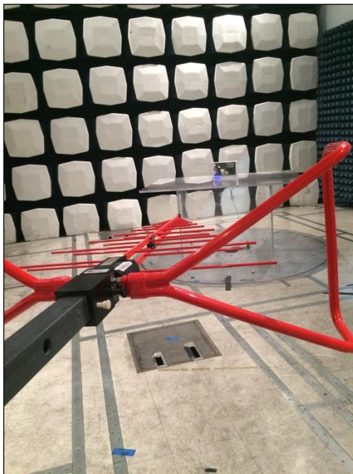
Photograph 1. Radiated Spurious Emissions, Test Setup, 30 MHz – 1 GHz
