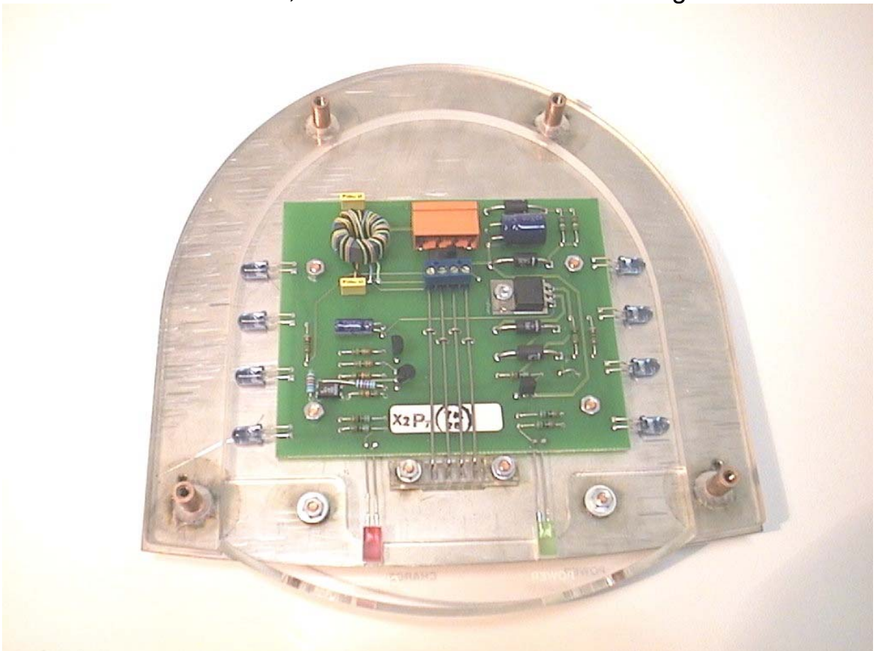
CS0188 touchCUE-SRF, internal bottom view into docking station
