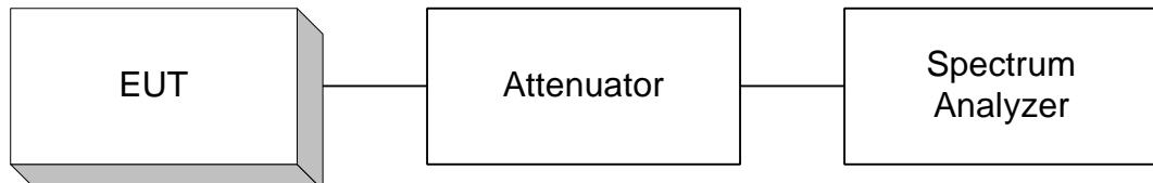
**Para. No. 2.991 Spurious Emissions at Antenna Terminals**
