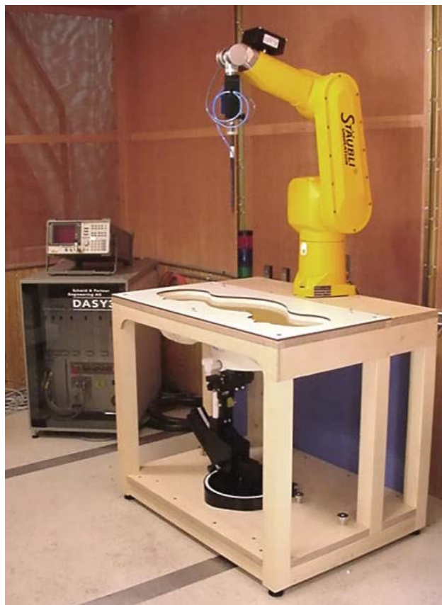
DASY3 SAR Measurement System with SAM phantom
