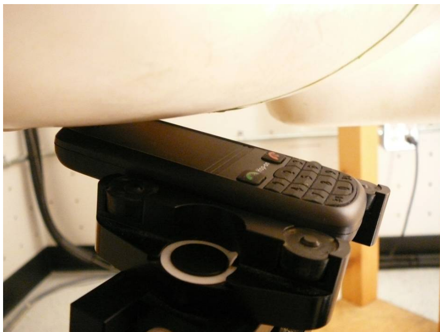
EUT Right Head Tilt Setup Photo
