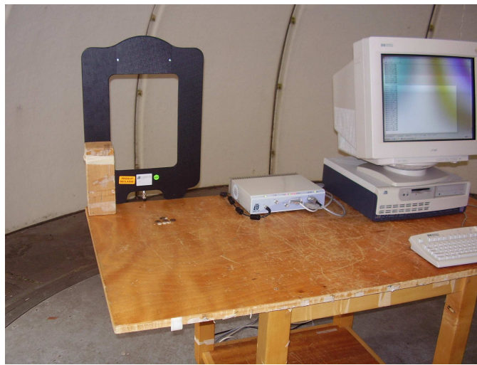
Radiated emission test setup (AERO-LB and AERO-LC antennas, in vertical position)
