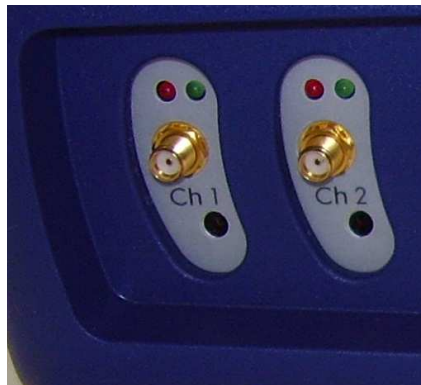
Detail view of SMA connectors (RF channels)
