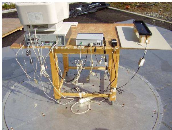
Radiated emission test setup
