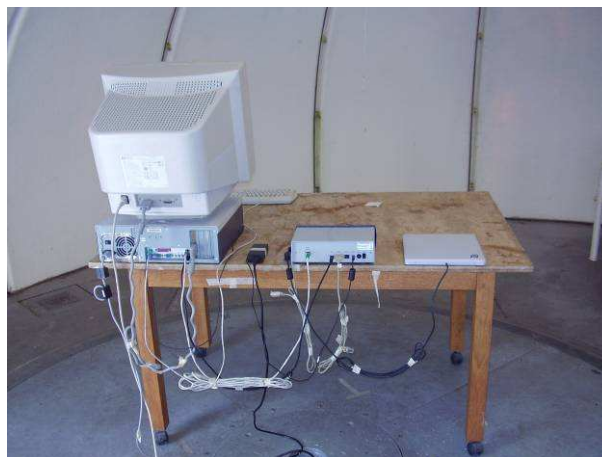
Radiated emission test setup (L-SA3, L-SA4, AERO-LI antenna in horizontal position)
