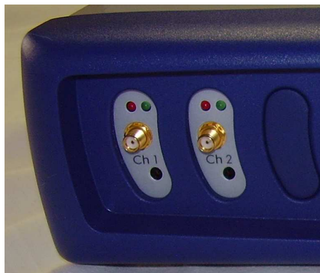
Detail view of SMA connectors (RF channels)
