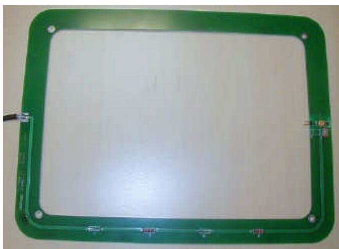
Internal view of one antenna, ferrite removed, component side
