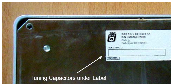
Figure 6: Position of the Tuning Capacitor on L-SA4 Antenna
