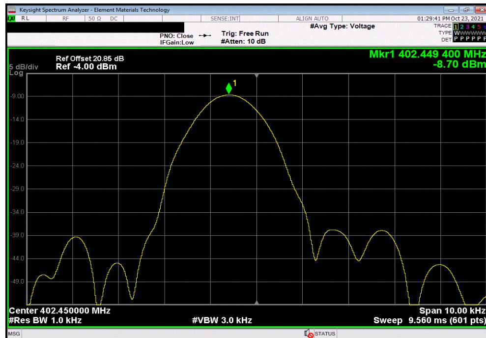
CW, Extreme Temperature +50°C, High Channel, 404.550 MHz
