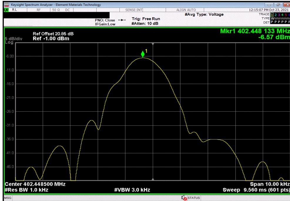
CW, Extreme Voltage -15%, 4.25 VDC High Channel, 404.550 MHz
