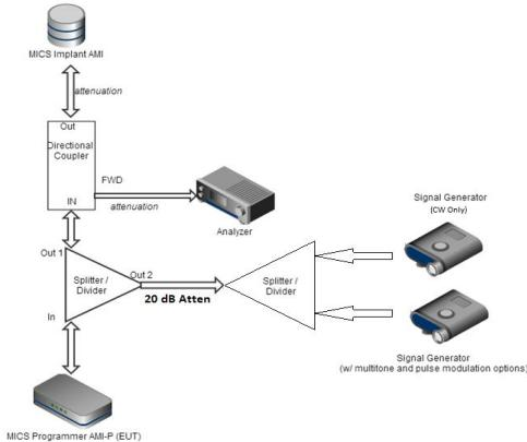
One signal generator was set to multi-tone operation to cause equal interference across the entire band. The amplitude of the multi-tone signals (out of operation region) were set to the LBT threshold of  $10 \times \text{LOG}(\text{Bandwidth}) - 150 + \text{Antenna Gain} + 10 \text{ dB}$ . The multi-tone generator was further configured to provide a least interfered channel (LIC) at amplitude of LBT threshold +3 dB.
