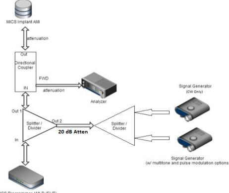
One signal generator was set to multi-tone operation to cause equal interference across the entire band except for the intended frequency (Fc). The second signal generator was configured to a CW signal on the intended frequency (Fc). The spectrum analyzer was set to zero span with a sweep time equal to 10 seconds.
