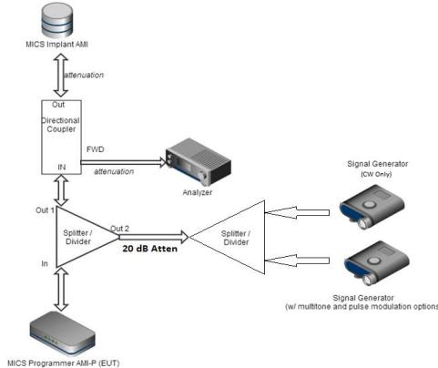
One signal generator was set to multi-tone operation to cause equal interference across the entire band. The amplitude of the multi-tone signals (out of operation region) were set to the LBT threshold of  $10 \times \text{LOG}(\text{Bandwidth}) - 150 + \text{Antenna Gain} + 10 \text{ dB}$ . The multi-tone generator was further configured to provide a least interfered channel (LIC) with amplitude set to the LBT threshold + 3 dB.
