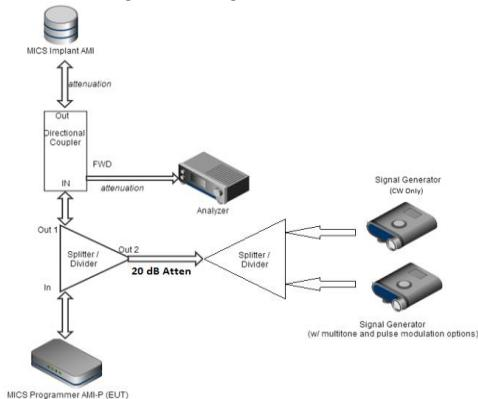
A signal generator was set to multi-tone operation to cause equal interference across the entire band, except one channel ( $F_c$ ) was left available. The multi-tone operation (out of operation region) was also set to Pulse modulation with a Period of 10 mS, and a Pulse Width of 0.1 mS. The second (CW only) signal generator was not used for this test, but remained in the test setup. The spectrum analyzer was set to measure the transmit band of 402-405 MHz.
