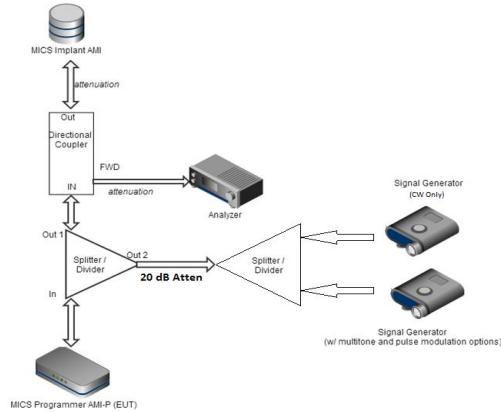
One signal generator was set to multi-tone operation to cause equal interference across the entire band except for the intended frequency ( $F_c$ ). The amplitude of the multi-tone signals (out of operation region) were set to the LBT threshold of  $10 \cdot \log(\text{Bandwidth}) - 150 + \text{Antenna Gain} + 3 \text{ dB}$ .
