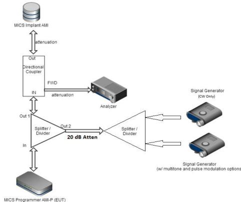
One signal generator was set to multi-tone operation to cause equal interference across the entire band except for the intended frequency ( $F_c$ ). The amplitude of the multi-tone signals (out of operation region) were set to 10 dB above the LBT threshold:  $10 \times \text{LOG}(\text{Bandwidth}) - 150 + \text{Antenna Gain} + 10 \text{ dB}$ . The multi-tone generator was further configured to provide a least interfered channel (LIC) at amplitude of LBT threshold +3 dB.
