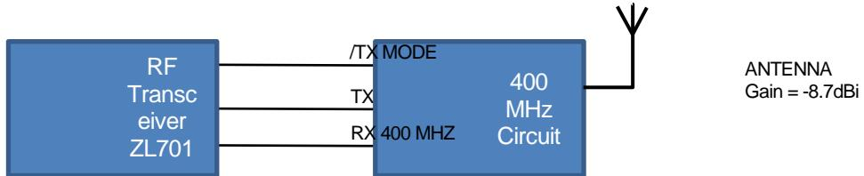
§ 95.2587 (a) The antenna associated with the MedRadio Transceiver is supplied with the Model 2100 Wireless Transmitter. Note: it is not possible to change the antenna. The device used during radio testing was manufactured under the current board assembly information version of the BSM06 (Base Station Module 06) which uses the abovementioned antenna.
