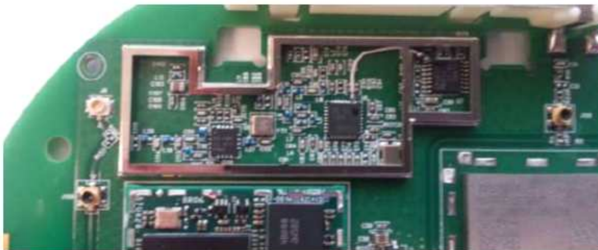
Figure 10: Internal Photo – 900MHz Radio Shield Removed
