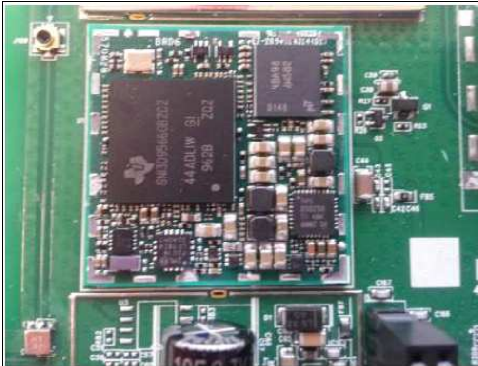
Figure 11: Internal Photo – ISOM Module U1 Shield Removed
