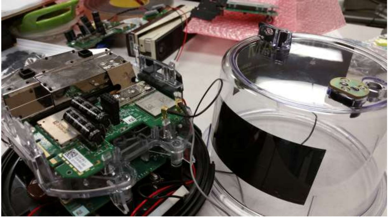
MODULE 574161 WAN ANTENNA POSITION SHOWN IN THE CONFIGURATION AS THEY WOULD BE MOUNTED IN THE HOST COVER
