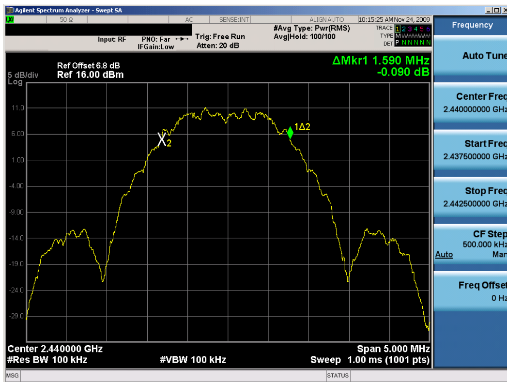
Plot 6-2. 6dB Bandwidth Plot (802.15.4 – Ch. 18)
