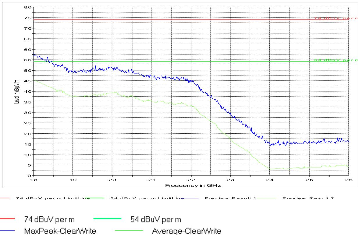
**6.5 Receiver Spurious Emissions- Radiated****6.5.1 Limits:**6.5.1.1 FCC CFR §15.1096.5.1.2 RSS-Gen
