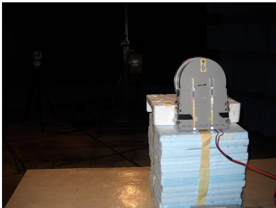
**Radiated Spurious Emissions Test Setup Pictures****30MHz – 1GHz**
