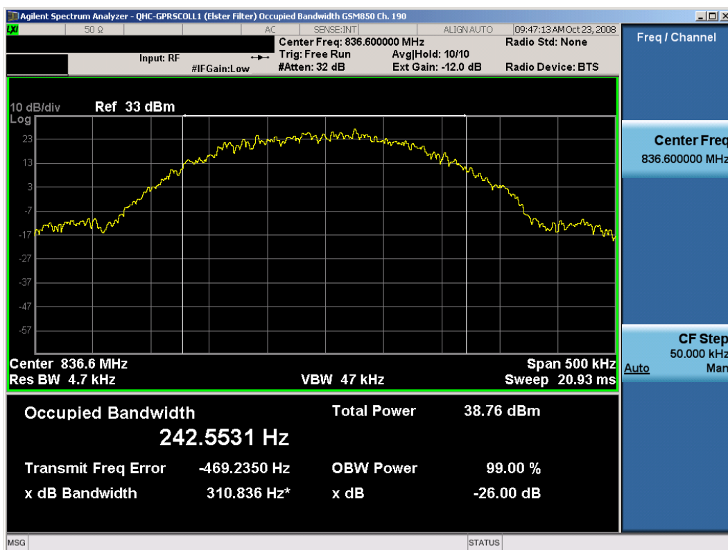
Plot 8-6. Occupied Bandwidth Plot (Cellular GSM Mode – Ch. 190) – Elster Filter
