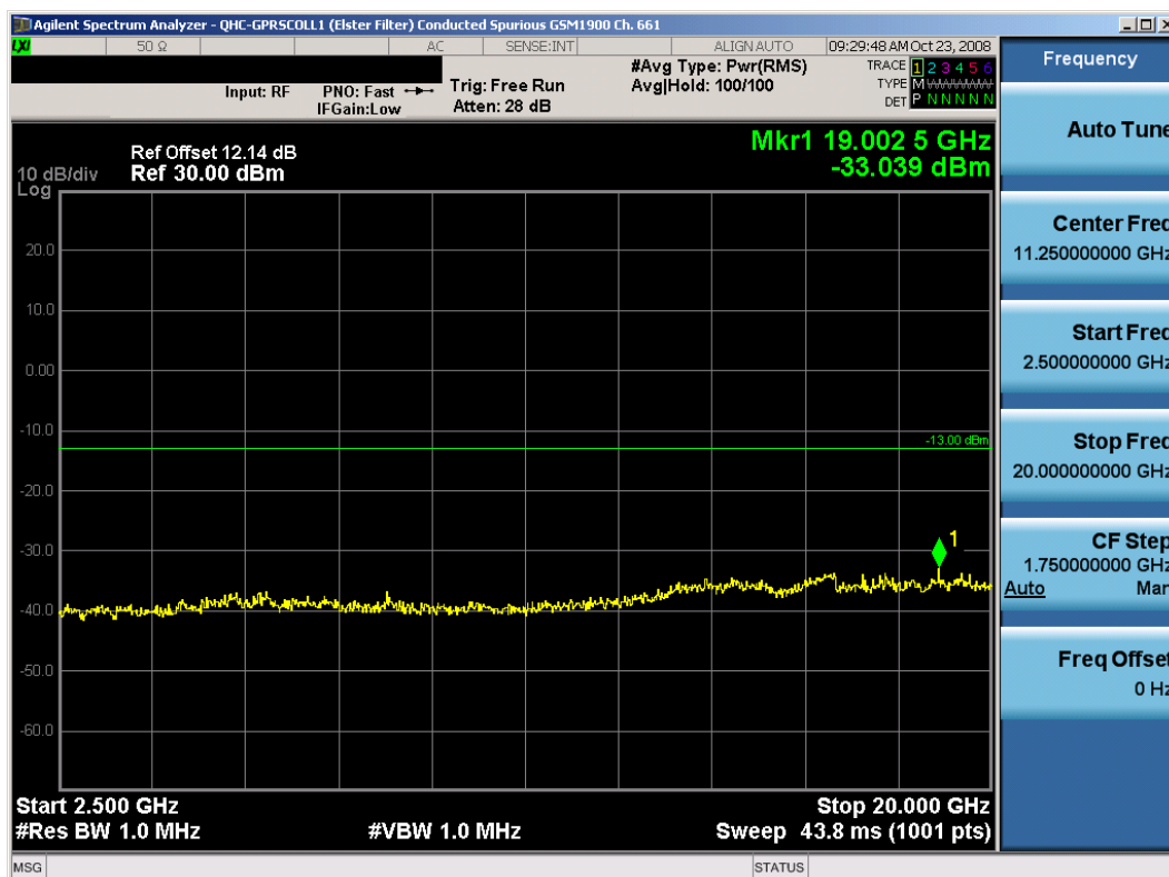
Plot 8-14. Conducted Spurious Plot (PCS GSM Mode – Ch. 661) – Elster Filter
