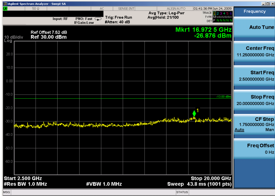
Plot 7-11. Conducted Spurious Plot (PCS GSM Mode – Ch. 512)
